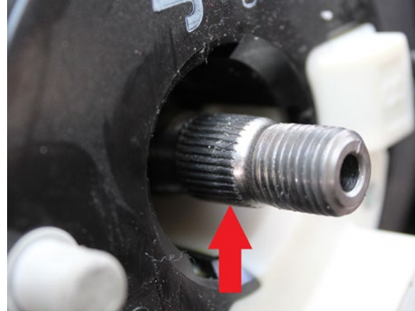
Figure 9. Steering column shaft damage, the 2010 Nissan Versa
