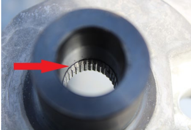
Figure 8. Steering wheel spline damage, the 2010 Nissan Versa
