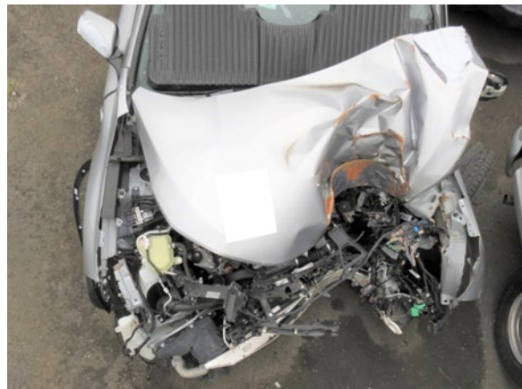
Figure 5. Front plane damage, the 2018 Honda CR-V Figure 6. Front plane damage, the 2018 Honda CR-V
