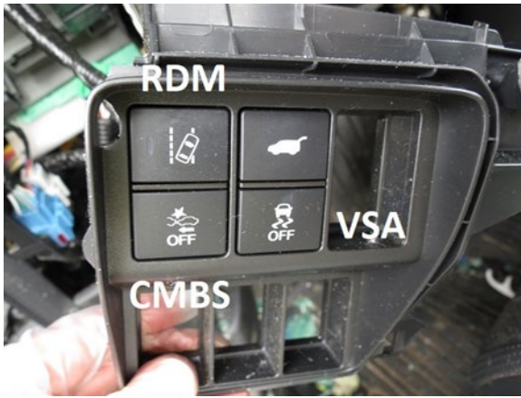
Figure 7. Crash avoidance technology controls, left instrument panel, the 2018 Honda CR-V
