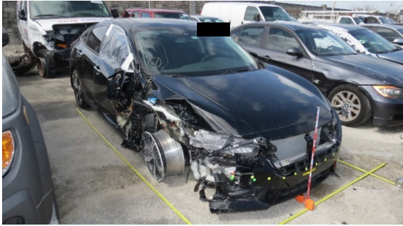
Figure 7. Front plane damage to the Honda as documented during the SCI vehicle inspection
