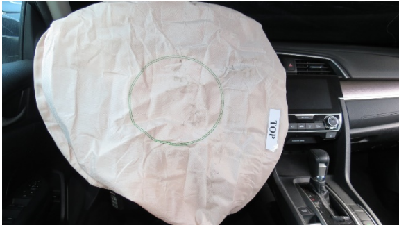
Figure 11. View of the deployed driver's frontal air bag in the Honda at the time of the SCI inspection
