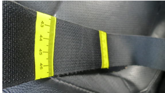
Figure 10. Latch plate loading evidence on the driver's seat belt system in the Honda
