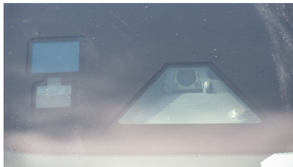
Figure 14. View of the Honda's optical sensor for the FCW and LDW systems
