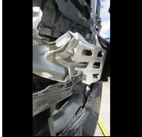
Figure 8. Front right corner of the Honda's reinforcement bar damage as documented during the SCI vehicle inspection
