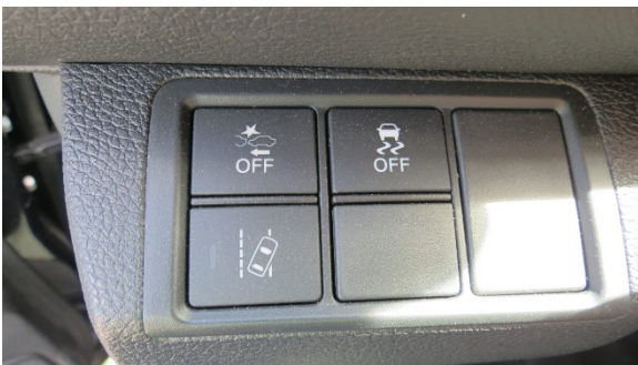
Figure 13. View of the Crash Avoidance System Buttons located on the instrument panel left of the steering column
