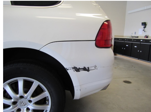
Figure 3. Sideswipe damage to the left aspect of the rear bumper fascia
