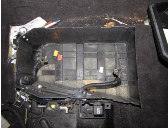
Figure 5. Overhead view of the battery well in the Porsche with the battery removed
