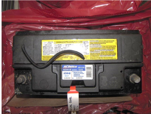
Figure 6. Image of the AC-Delco 60 series Group 49 12-volt battery found in the Porsche
