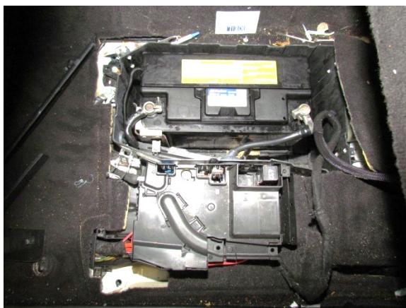
Figure 4. Battery positioned in the well under the driver's seat
