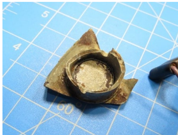
Figure 8. Air bag inflator “booster tube” fragment, the 2004 BMW 325i
