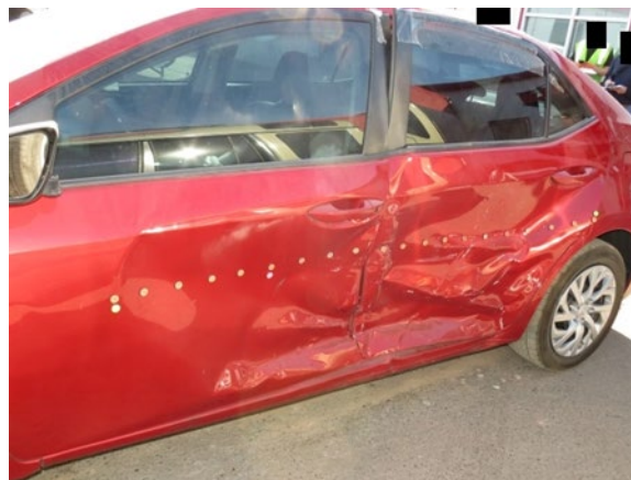
Figure 9. Left plane damage, the 2018 Toyota Corolla
