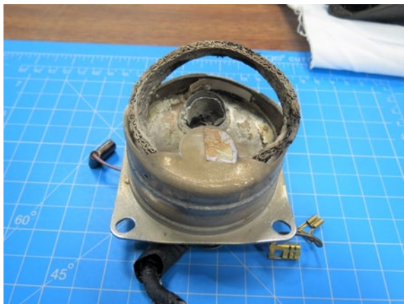
Figure 7. Ruptured air bag inflator, the 2004 BMW 325i
