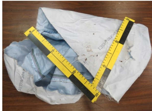
Figure 6. Deployed driver's frontal air bag, the 2004 BMW 325i
