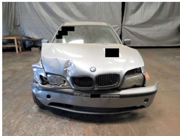
Figure 4. Front plane damage, the 2004 BMW 325i
