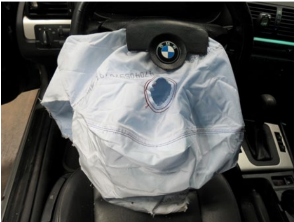
Figure 5. Deployed driver's frontal air bag, the 2004 BMW 325i
