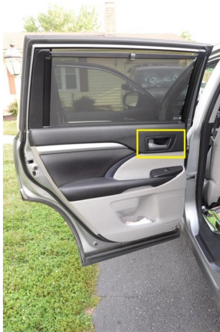
Figure 7. Left rear door panel documenting the door release lever, the lock lever, and the sun shade (Image provided by the investigating police department.)
