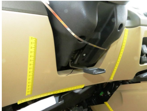
Figure 6. Driver knee contact to the left lower instrument panel in the Honda
