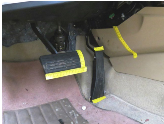
Figure 9. Brake pedal (left) and accelerator pedal (right) with the original floor mat and secondary aftermarket floor mat in the Honda at the time of the SCI vehicle inspection
