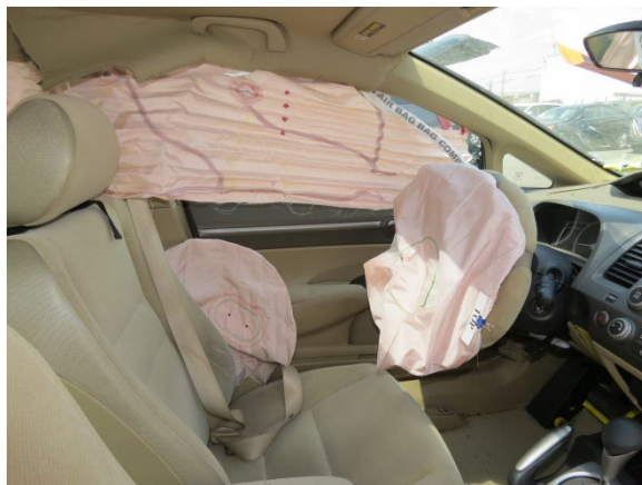
Figure 8. Deployed supplemental restraint systems in the Honda at the time of the SCI vehicle inspection
