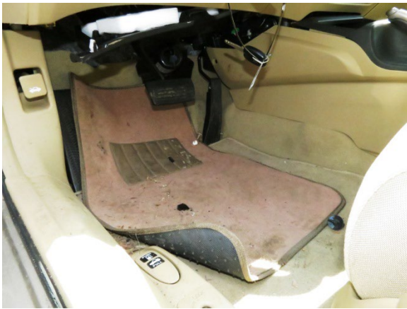
Figure 10. Aftermarket floor mat in the Honda, positioned undisturbed at the onset of the SCI vehicle inspection
