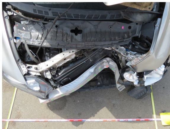
Figure 5. Overhead view of the damage profile to the Honda's front plane associative to the Event 5 impact
