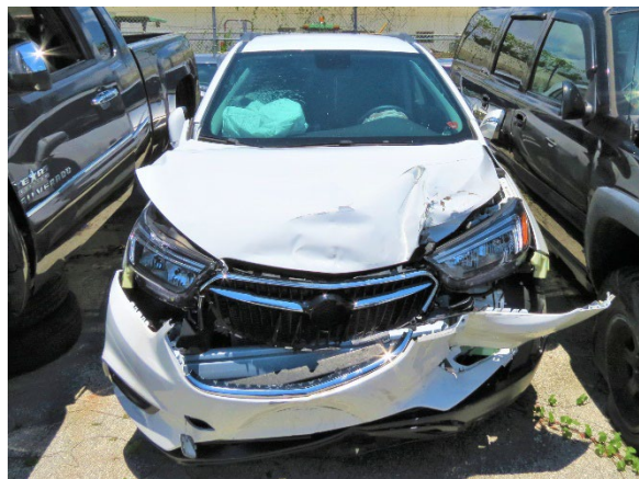
Figure 24. Front-plane view of the damage profile to the 2017 Buick Encore
