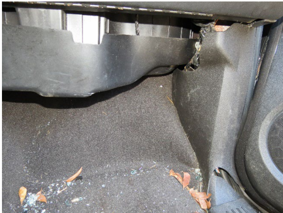
Figure 10. Visible longitudinal intrusion of the floor/toe pan at the Chevrolet's front-row right position
