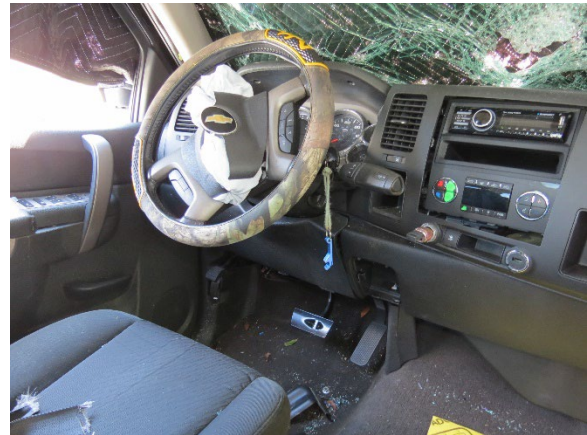
Figure 11. Front components within the Chevrolet at the driver's seat position
