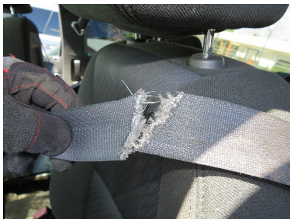
Figure 12. Upper cut point to the shoulder portion of the driver's seat belt system within the Chevrolet
