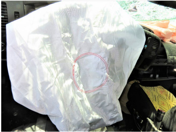
Figure 14. Deployed driver's frontal air bag within the Chevrolet
