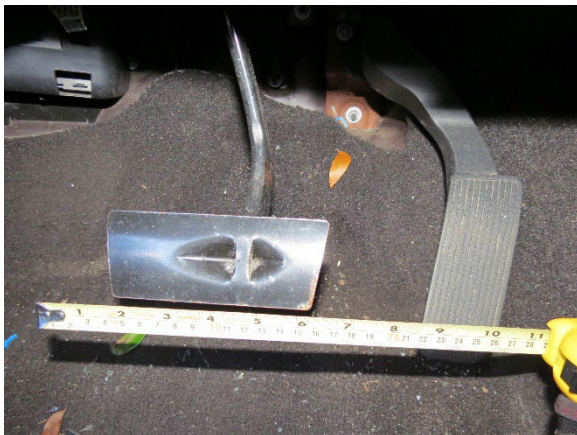
Figure 17. View of the driver foot controls within the Chevrolet, depicting their size and separation
