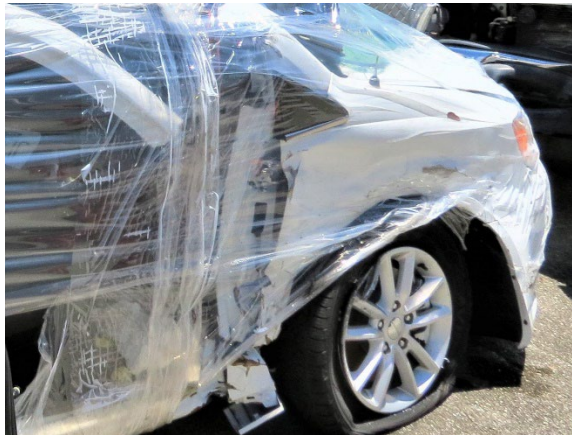
Figure 22. Damage pattern to the right plane of the Dodge from the impact with the Buick
