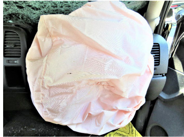
Figure 15. Deployed passenger's frontal air bag within the Chevrolet
