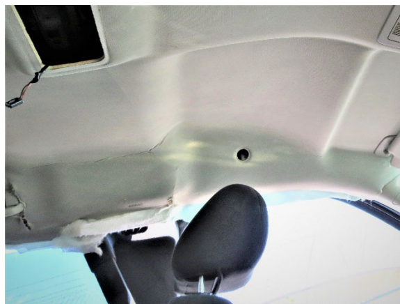
Figure 16. Remnants of the left IC air bag visible along the left-roof side rail of the Chevrolet
