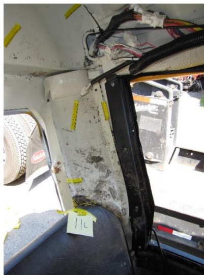
Figure 19. Blood and hair evidence observed at the left M-pillar of the school bus
