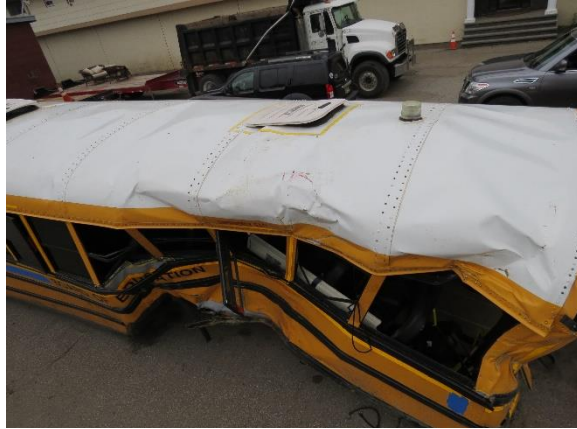
Figure 9. Overhead view showing the left plane deformation of the school bus body and red paint transfer on the roof
