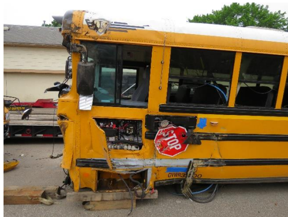
Figure 10. Left side view of the bus body showing damage attributed to Event 2
