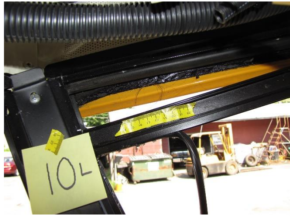
Figure 21. Hair observed at the junction of the left upper window and side rail at row 10
