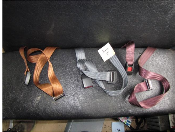
Figure 18. Observed condition and adjustment of the seat belts at row 1 left seat
