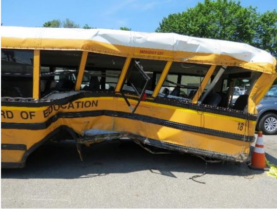
Figure 8. Left side view of the school bus body deformation
