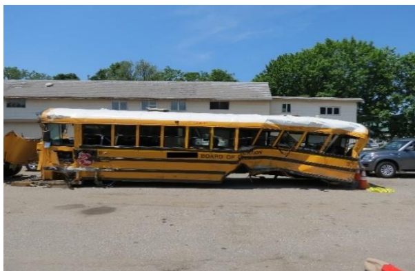
Figure 6. Left side view of the school bus body showing the location of the deformation and locations of the impacts (Events 1, 2, and 3)
