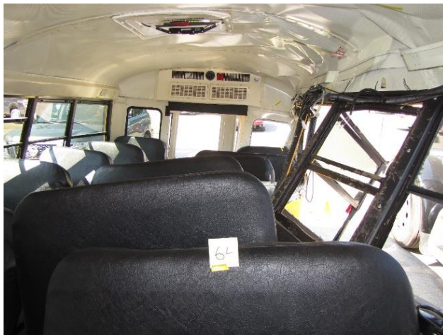
Figure 16. Rear-looking view of the bus interior showing the maximum intrusion at row 8 of the school bus
