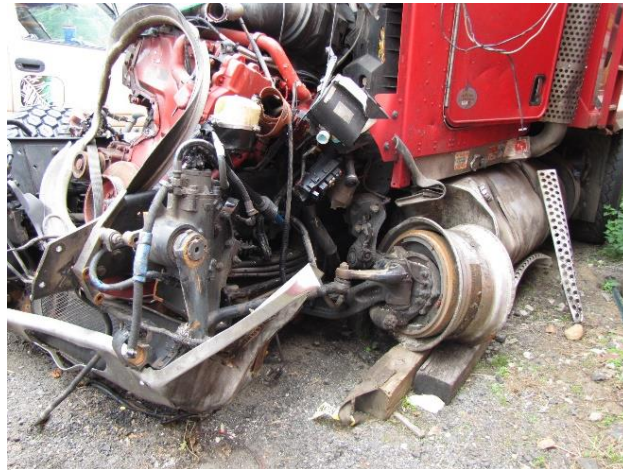
Figure 24. View showing the left plane damage of the Kenworth that extended rearward to the tag axle
