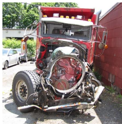
Figure 23. Front view showing the impact damage of the Kenworth
