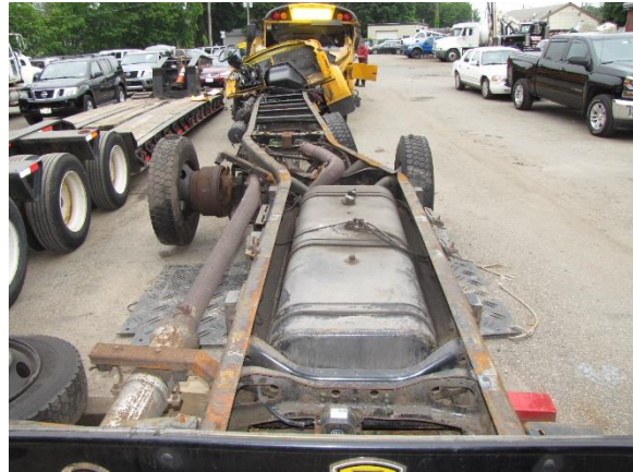
Figure 12. Forward-looking longitudinal view of the deformed bus ladder frame
