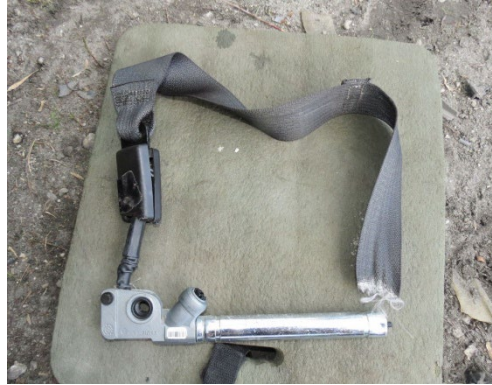
Figure 11. Post-crash status of driver's seat lower anchor pretensioner, lap webbing fractured
