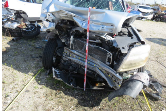
Figure 7. Frontal damage to the GMC
