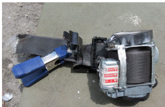
Figure 13. Close-up view of the driver's retractor removed from the GMC
