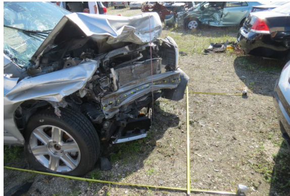
Figure 8. Right lateral view documenting the extent of crush to the GMC
