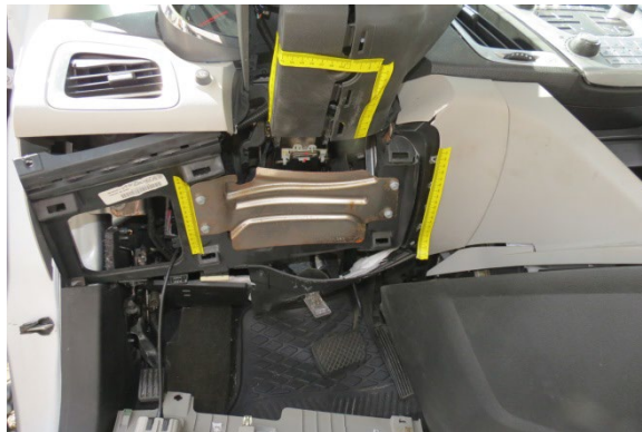
Figure 10. Driver knee contact evidence and damage to the lower steering column cover and knee bolster backer panel
