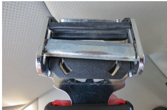
Figure 12. Close-up view of the GMC driver's lightweight locking latch plate
