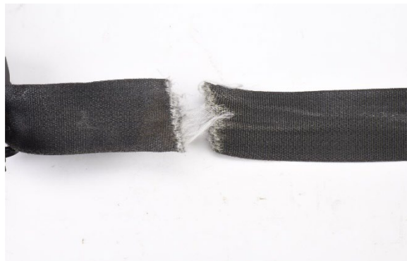
Figure 14. Tensile fracture of the lap belt webbing. Image taken during VRTC inspection
