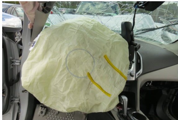
Figure 15. Deployed GMC driver's frontal air bag
