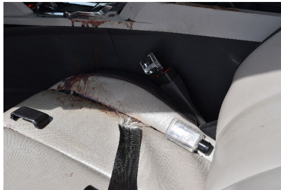
Figure 1. View of the buckled latch plate and portion of the separated webbing of the GMC driver's seat belt system (image provided to NHTSA by the investigating law enforcement agency)
