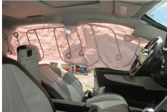
Figure 16. Deployed GMC left IC air bag
