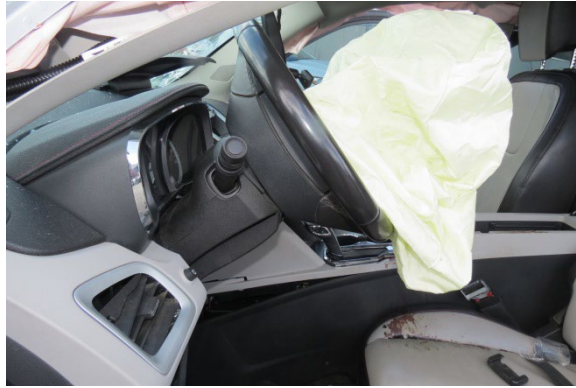
Figure 9. Bending of the steering wheel flange from driver loading
