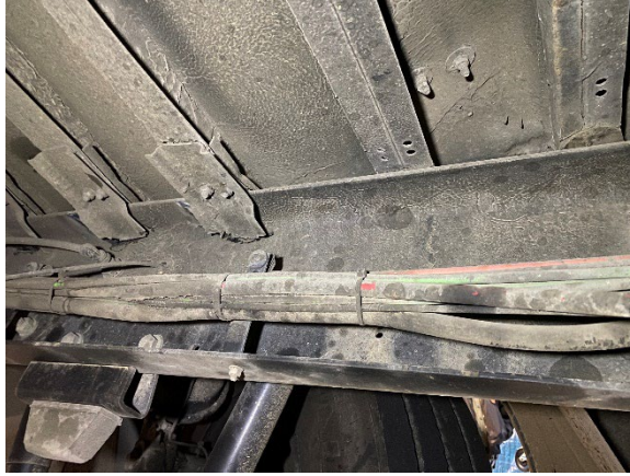
Figure 7. Right frame rail at RF wheel, ribs with and without flanges
