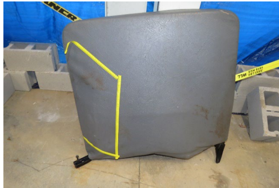
Figure 13. Padded partition between the driver's seatback and the first row, left seat
