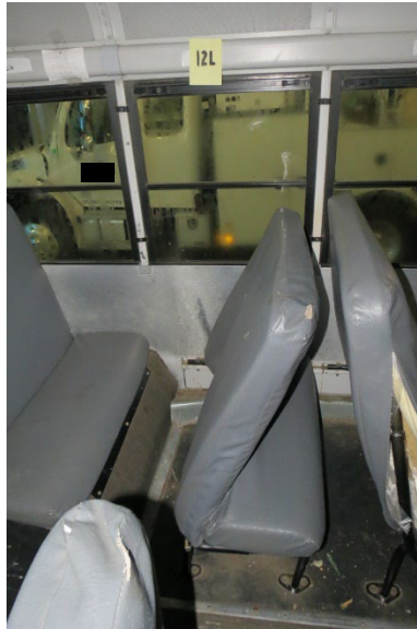
Figure 14. Damage to row 12 left seatback from row 13 left occupant contacts
