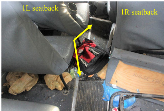
Figure 9. On-scene police image showing lateral lines of floor buckling at driver's seat and second row
