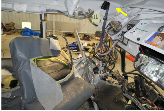
Figure 11. Intrusion to the driver area and the first row (note the proximity of bulkhead to the shoulder belt D-ring anchor compared to the exemplary in Figure 12)
