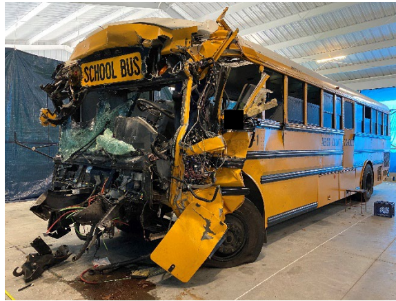
Figure 6. Front plane damage of the bus
