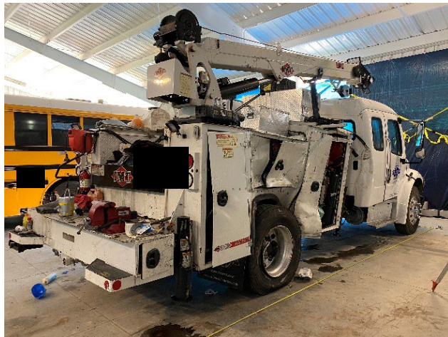
Figure 16. The Freightliner, right plane damage (rear half)
