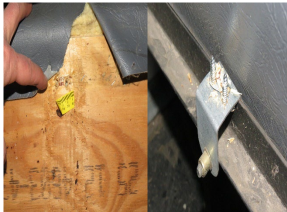
Figure 15. Holes (L) on the bottom of the seat cushion that tore away from the bracket (R)
