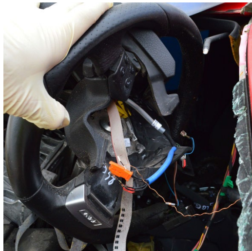
Figure 17. Law enforcement image of the steering column and damaged electrical wiring/connectors
