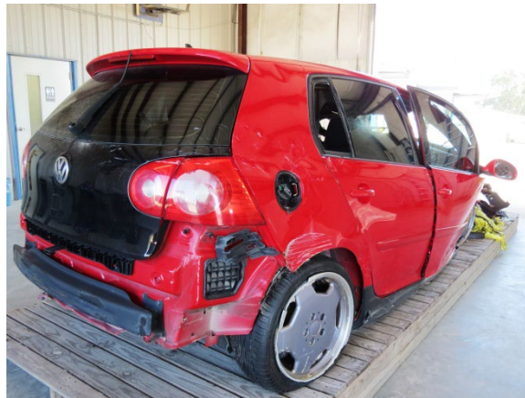
Figure 8. Right-rear oblique view of the Volkswagen's Event 3 damage, overlapped by damage from Event 5
