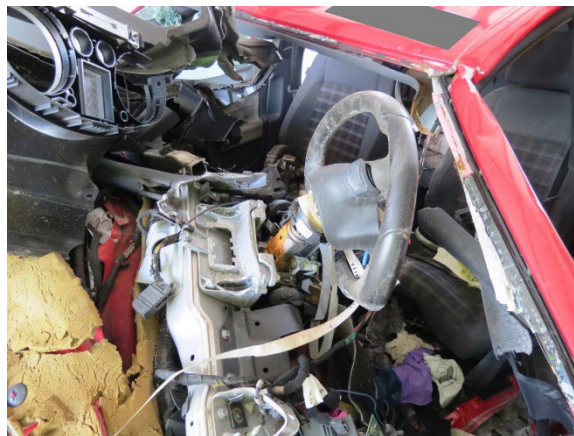
Figure 13. View of the Volkswagen's displaced and severely damaged steering column
