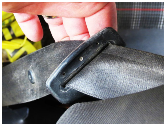
Figure 14. Heavy loading evidence visible in the belt path of the Volkswagen driver's seat belt latch plate
