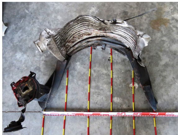
Figure 11. Overhead view of the deformed and separated bumper beam, with the crush measurement gauge
