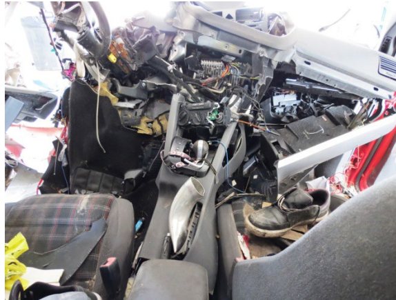
Figure 12. Forward-facing view of the Volkswagen's intruded and heavily damaged instrument panel
