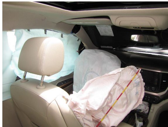
Figure 12. Oblique interior view showing the deployed air bags at the driver's position
