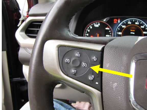
Figure 14. Interior view of the GMC's steering wheel and the operational pad for the cruise control
