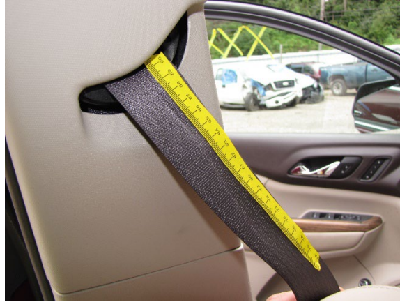
Figure 11. GMC interior image showing the crease in the driver's shoulder belt webbing at the left D-ring
