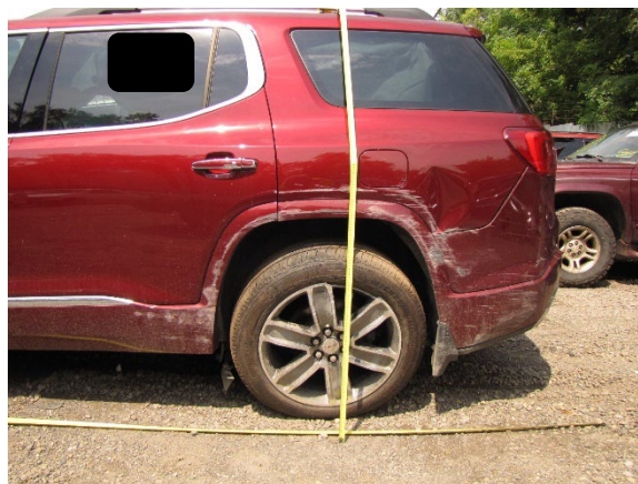
Figure 9. Left view of the GMC's Event 2 damage
