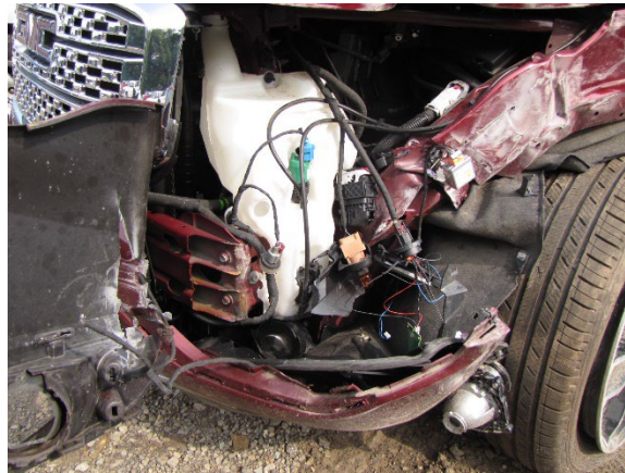
Figure 8. Close-up view of the minimal damage at the left end of the GMC's front bumper reinforcement
