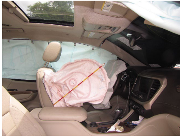
Figure 13. Right interior view of the GMC's front row and the deployed air bags
