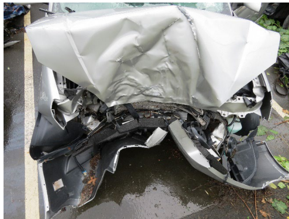
Figure 8. Front-plane damage profile to the Chevrolet
