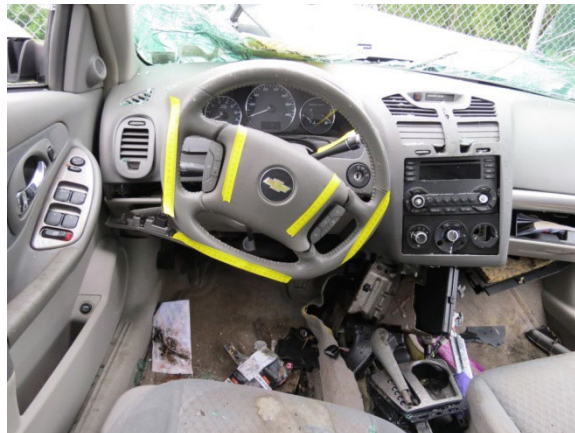
Figure 10. Driver trajectory and loading damage to the steering assembly and the lower instrument panel
