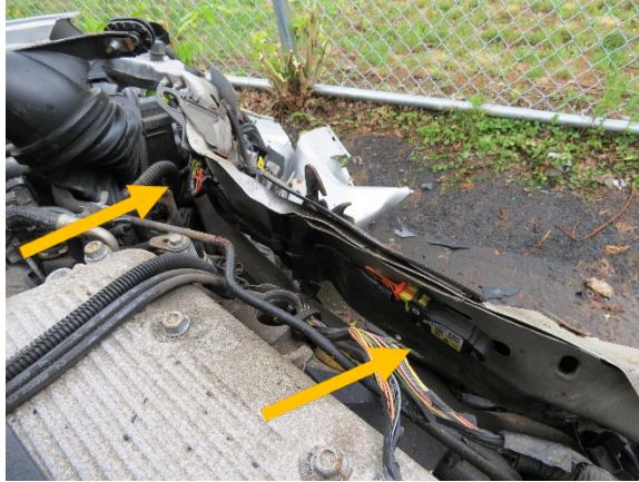
Figure 13. Satellite crash sensors mounted to the radiator support
