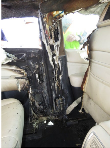
Figure 2. Interior view of the left B-pillar area and the fire damage
