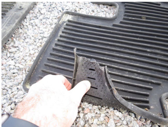
Figure 10. View of the Infiniti's OEM second row rubber floor mat damaged by the fire
