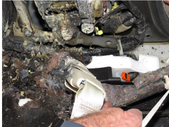
Figure 25. Interior image showing the left lower anchor and fire damage in the Infiniti
