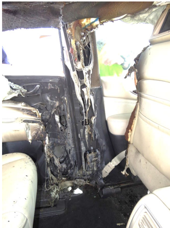
Figure 12. Overall view of the Infiniti's fire damage
