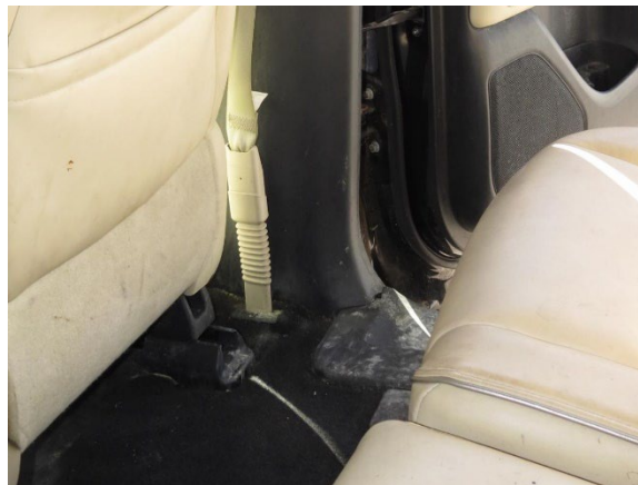
Figure 22. Interior image showing the right lower anchor pretensioner prior to its removal from the involved Infiniti
