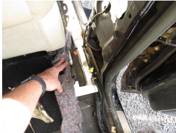
Figure 23. Interior view of the Infiniti's right lower anchor pretensioner location
