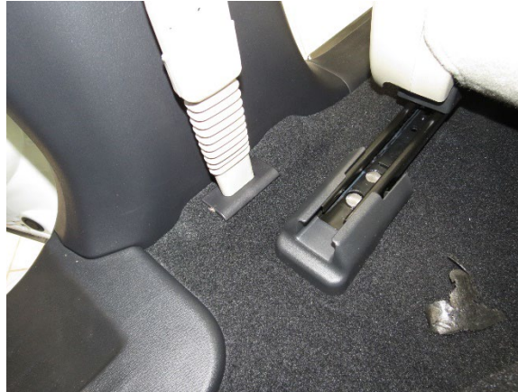
Figure 21. Interior view of the left lower anchor pretensioner location in an exemplar Infiniti
