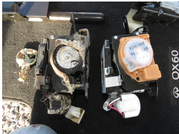
Figure 19. Image showing the left and right retractor pretensioners (aft surface shown) removed from the Infiniti
