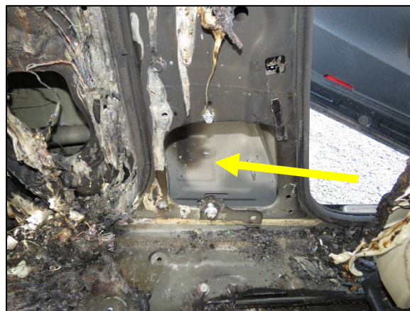
Figure 16. Image showing the Infiniti's left B-pillar cavity, discoloration in the cavity and aft of the retractor location
