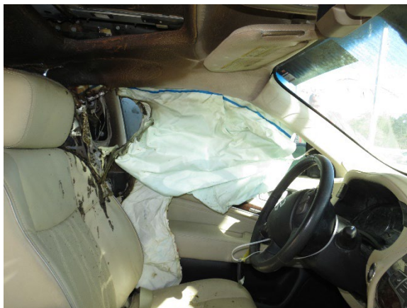
Figure 6. Lateral view of the Infiniti's deployed left seat-mounted side impact and IC air bags
