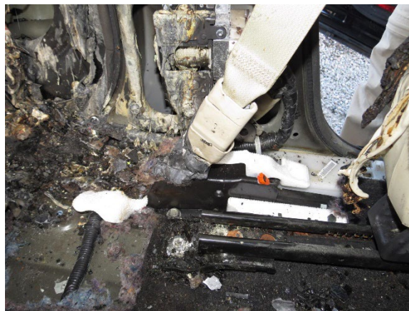
Figure 24. Interior image showing the left lower anchor and fire damage in the Infiniti
