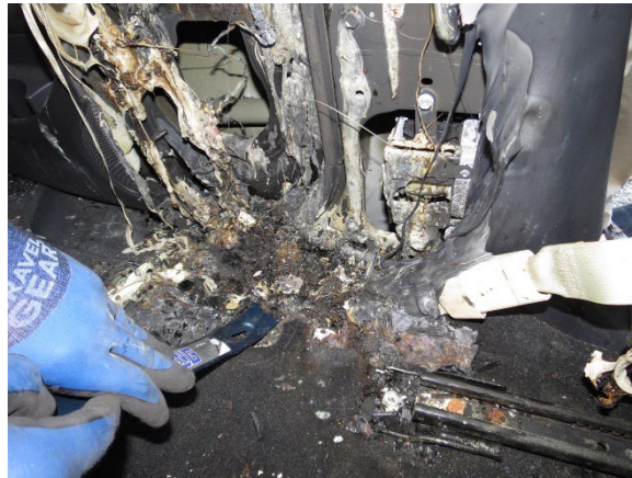
Figure 13. Close-up view of the fire debris and damage at the base of the Infiniti's B-pillar
