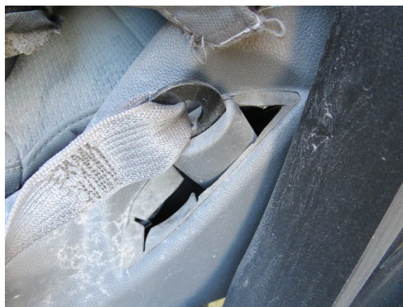
Figure 11. View of the Chevrolet driver's lower anchor visibly drawn into the fascia by pretensioner actuation
