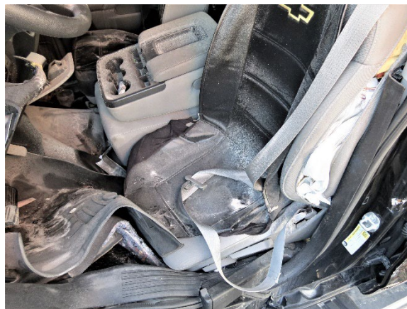
Figure 10. Chevrolet driver's seat belt system at the time of the SCI vehicle inspection
