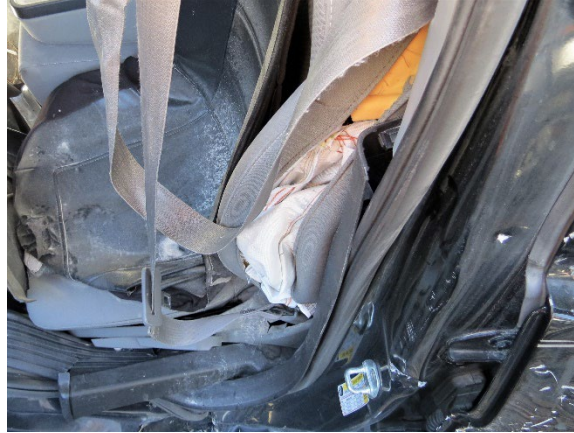
Figure 12. Deformed driver's seat engaged against the intruded left sill and B-pillar of the Chevrolet
