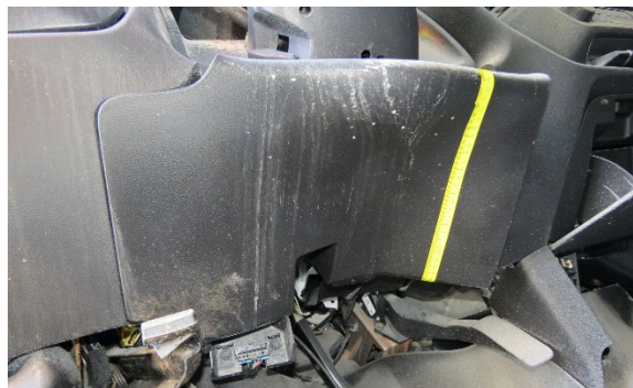
Figure 9. Occupant contact to the Chevrolet's left lower instrument panel from the driver's knees
