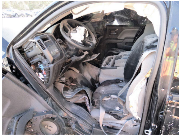
Figure 7. View of the intruded components surrounding the driver's position of the Chevrolet
