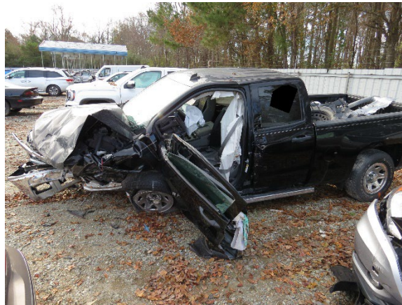
Figure 5. Front plane damage and left wheelbase reduction to the Chevrolet
