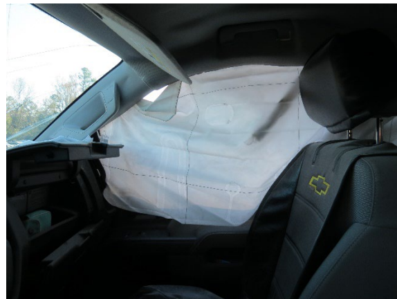
Figure 16. View of the Chevrolet's deployed right IC air bag, forward aspect, at the time of the SCI inspection
