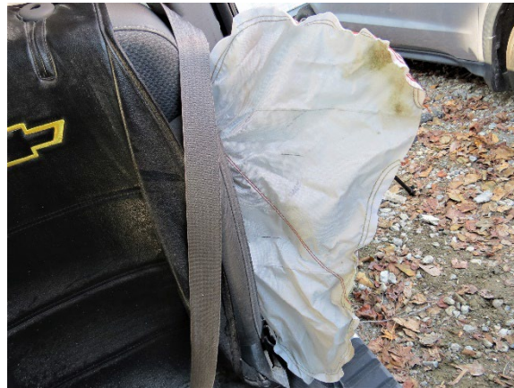
Figure 14. Chevrolet driver's deployed seat-mounted side impact air bag
