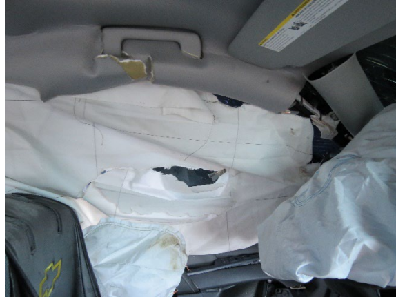
Figure 15. View of the Chevrolet's left IC (cut forward aspect), left seat-mounted, and driver's frontal air bags
