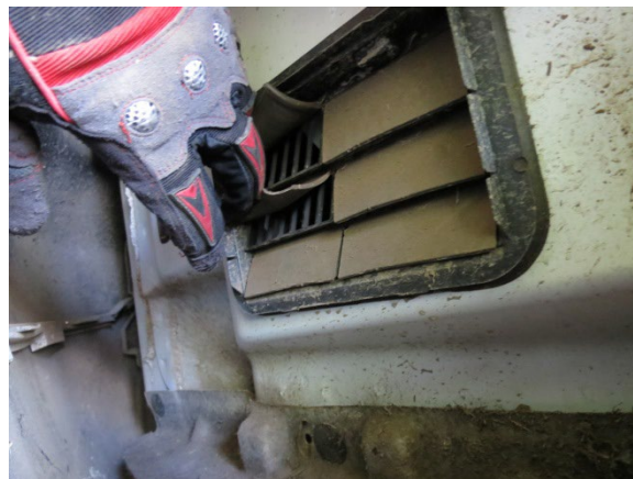
Figure 11. View of the Ford's right rear air extractor
