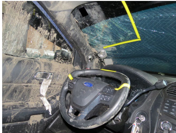
Figure 9. Driver contact to the steering wheel rim and windshield with the Ford
