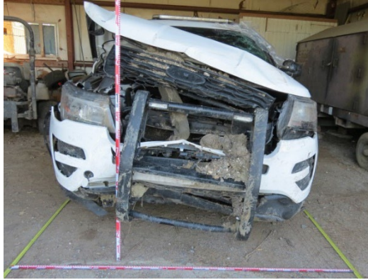
Figure 6. View of the Ford's front plane damage
