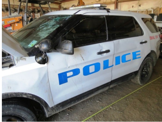
Figure 8. Minimal damage to the Ford's left plane
