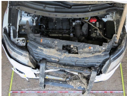
Figure 7. Overhead view of the Ford's front plane damage profile
