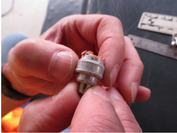
Figure 14. Top view of gas generator
