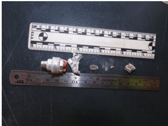
Figure 9. LF pretensioner gas generator and shrapnel removed from left-rear passenger's leg
