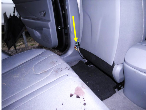
Figure 8. Holed left B-pillar
