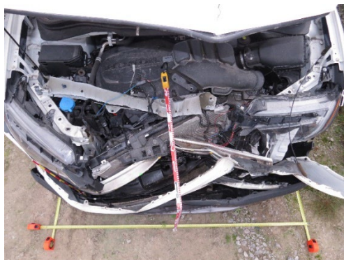
Figure 21. Overhead view of the Honda's overlapping frontal damage
