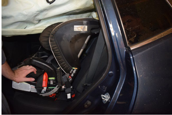
Figure 10. Installed Britax CRS in the second-row left position of the Nissan. Image obtained from the investigating police agency.
