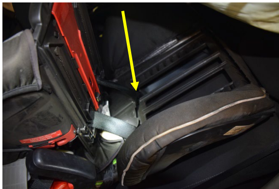
Figure 11. Separation of the Britax CRS shell and the horizontal fracture at the bottom of the harness adjustment mechanism. Image provided by the investigating police agency.
