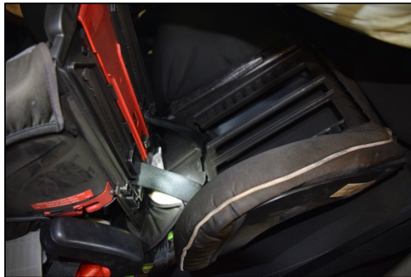
Figure 14. Fractured seat back of the Britax CRS and the altered position of the integral harness. Image provided by the investigating police department.
