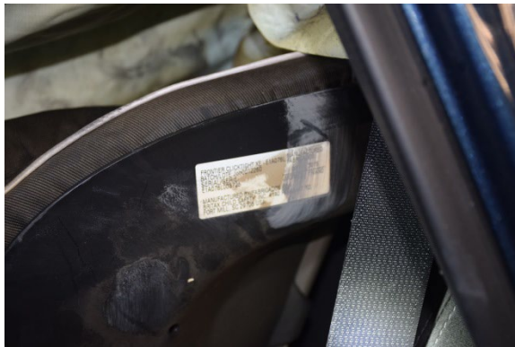
Figure 12. IC abrasions to the shell of the Britax CRS. Image provided by the investigating police agency.
