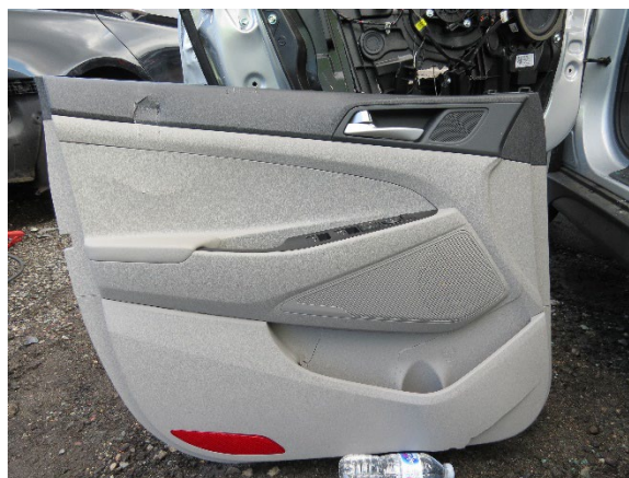
Figure 7. View of the Hyundai's driver door panel, devoid of discernable contact evidence
