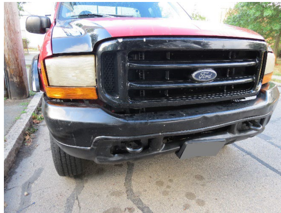
Figure 9. View of the Ford's front plane with minor direct contact discernable on the bumper beam
