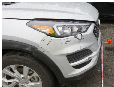
Figure 6. Minor right front corner damage to the Hyundai
