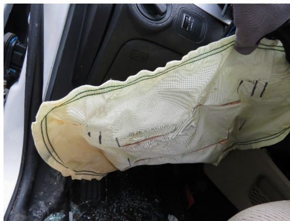
Figure 23. View of the Dodge's deployed driver knee air bag
