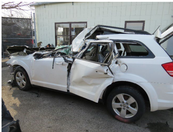
Figure 15. Left plane view of the Dodge and the severe deformation to the greenhouse/occupant compartment
