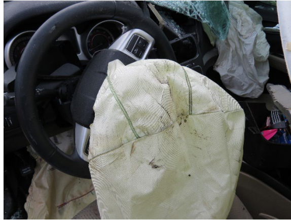
Figure 22. View of the deployed driver's frontal air bag in the Dodge
