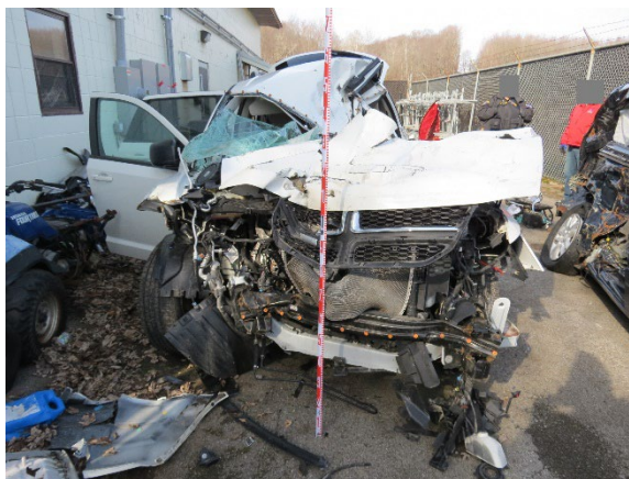
Figure 16. Front plane view of the Dodge and its damage profile
