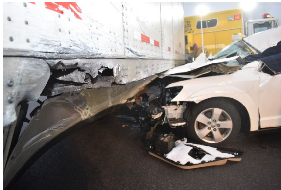
Figure 13. Close-up of the direct contact to the Wabash's left sill from the left pillar(s) of the Dodge (on-scene law enforcement image)
