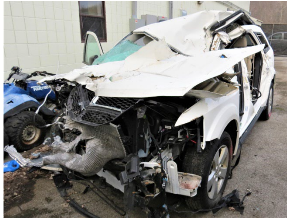
Figure 14. Left front oblique view of the Dodge at the time of the SCI vehicle inspection
