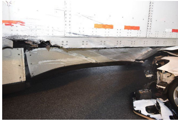
Figure 12. Damage pattern to the Wabash from the left plane underride impact by the Dodge (on-scene law enforcement image)
