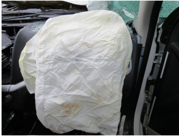
Figure 24. Passenger's frontal air bag deployed in the Dodge at the time of the SCI vehicle inspection
