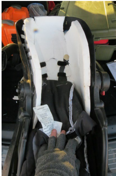
Figure 18. View of the fractured liner in the CRS
