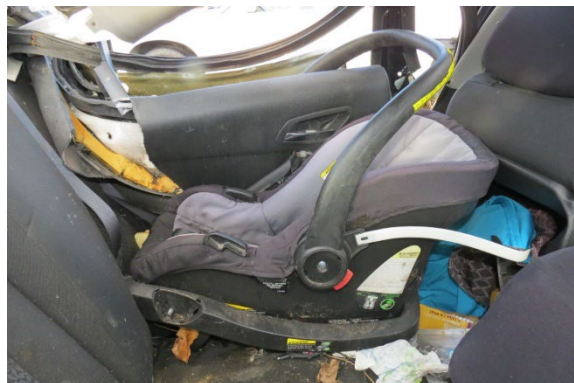
Figure 13. View of the CRS and intruded left rear door
