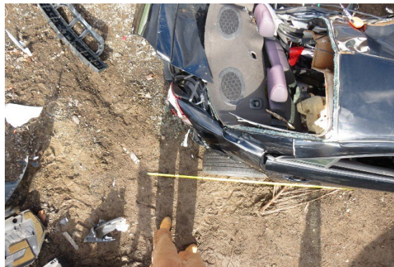
Figure 9. Overhead view of the Pontiac's right plane deformation
