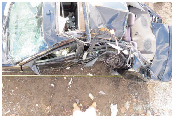
Figure 8. Overhead view of the Pontiac's left plane deformation
