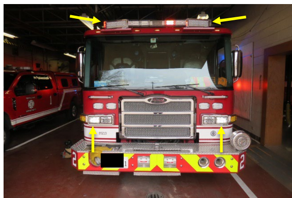
Figure 10. Front of the engine unit with arrows indicating flashing lights (some top bar lights are obscured by flood lights)
