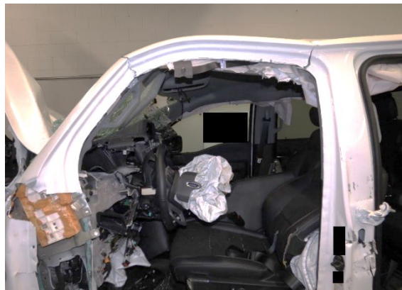
Figure 12. Buckling of the Ford's A and B pillars
