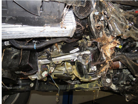
Figure 21. View of the Ford's steering rack with the front cross-member removed
