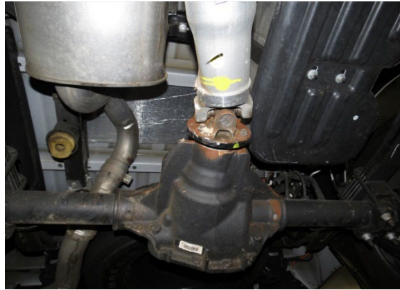
Figure 7. Damage from Event 3 (mound versus coupling)
