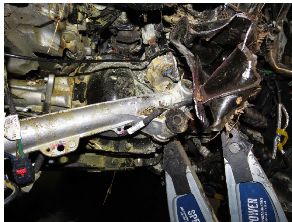
Figure 22. Hydraulic spreaders used to release tension and allow the steering rack removal
