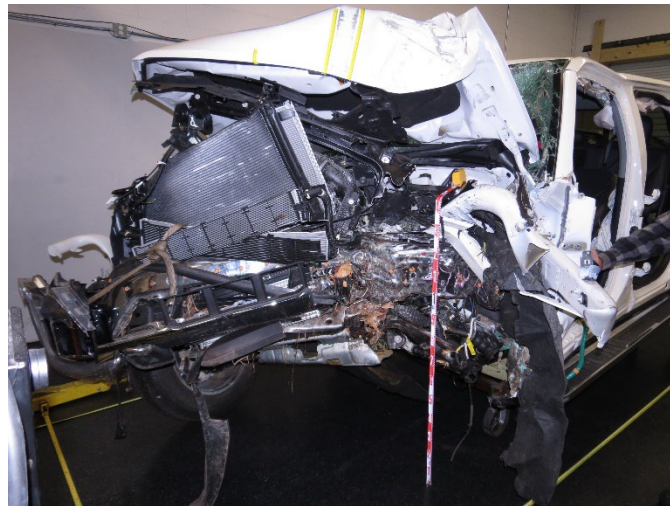
Figure 11. Left front oblique view of damage from Event 5
