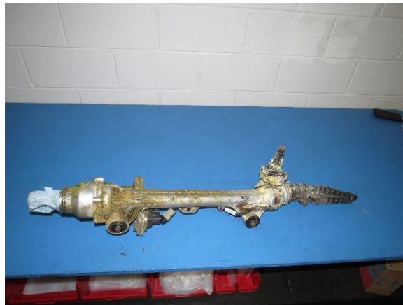
Figure 23. Steering rack after removal from the Ford
