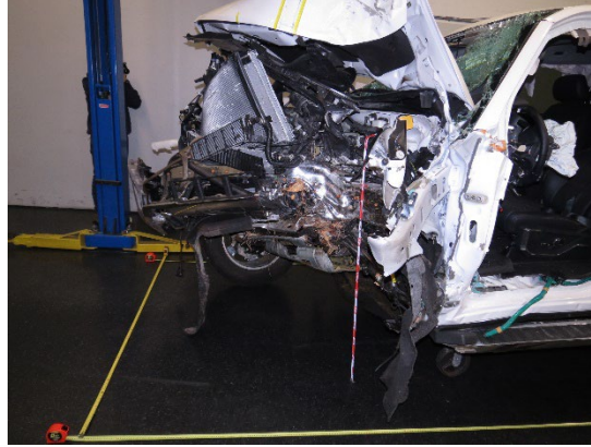
Figure 9. Lateral view of the direct damage from Event 5
