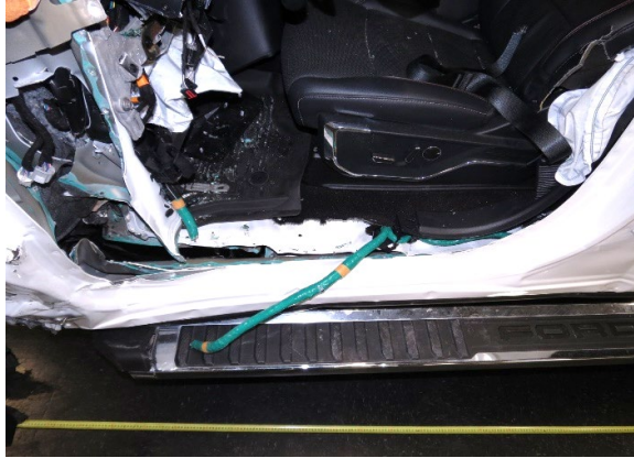
Figure 13. Driver door sill weld separation
