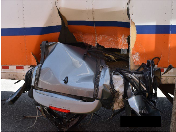
Figure 20. Right view of the trailer damage (On-scene police image)
