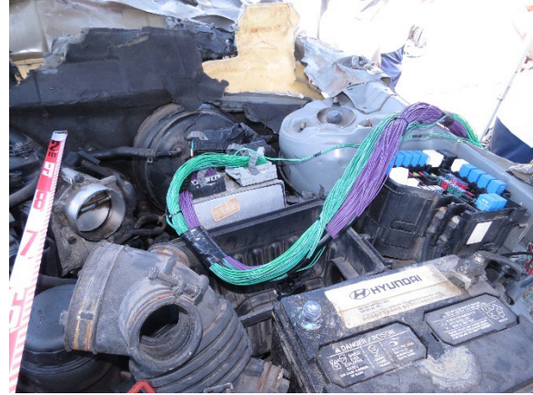
Figure 13. Image of the Hyundai's PCM during the proprietary imaging
