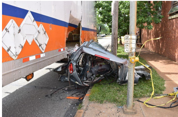
Figure 10. The separated greenhouse of the Hyundai removed from trailer (On-scene police image)
