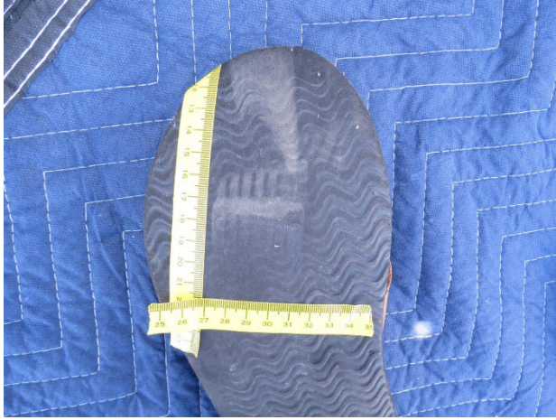
Figure 17. The driver's right footwear with pedal imprint
