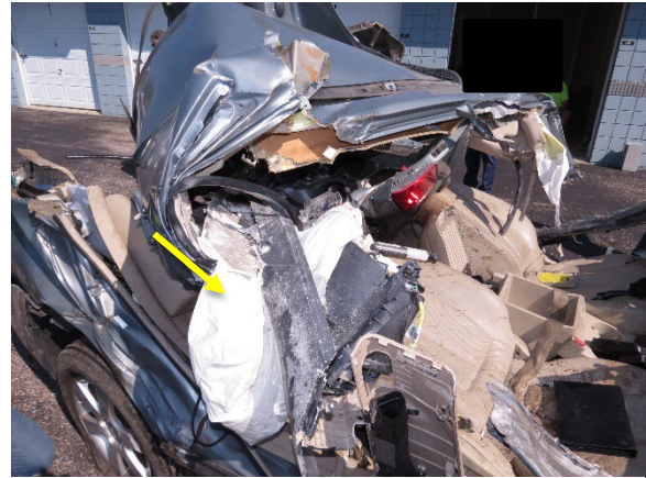
Figure 15. Image of the Hyundai's deployed passenger's frontal air bag separated from the instrument panel
