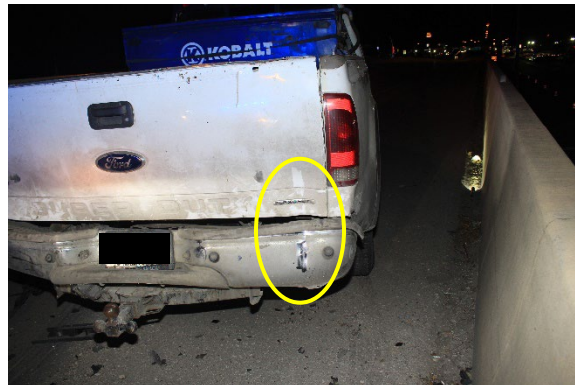
Figure 9. Police image, back plane, right aspect, damage from contact with the push-bar of the 2017 Explorer
