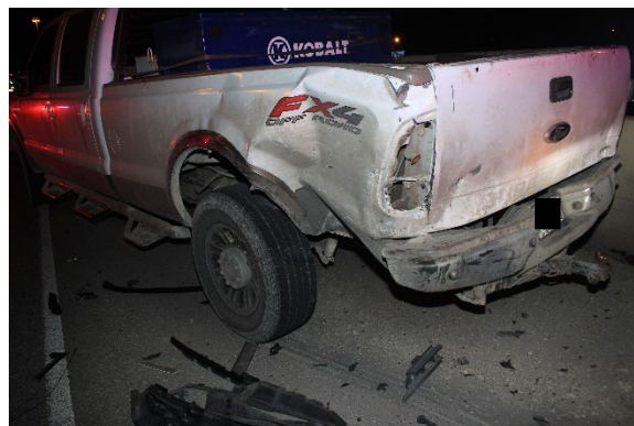
Figure 10. Police image, back and left plane damage from impact with the Chevrolet
