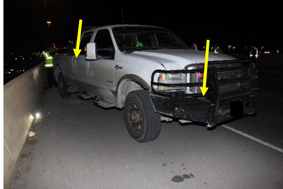
Figure 11. Police image, front right oblique view of the Ford F-250 and the probable area of non-motorist contact (Events 7 & 8)
