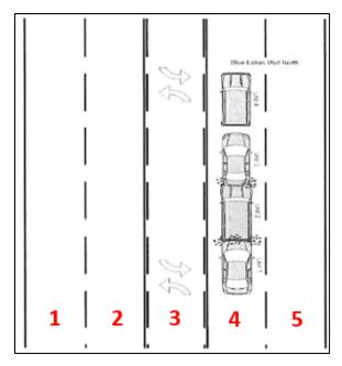
Figure 27. Example of counting lanes in a trafficway with a continuous left-turn lane
