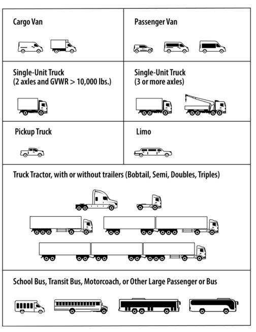
Figure 17. Motor vehicle body type examples
