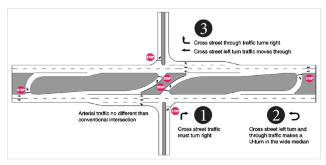
Figure 10. Example of an unsignalized RCUT intersection. Source: FHWA
