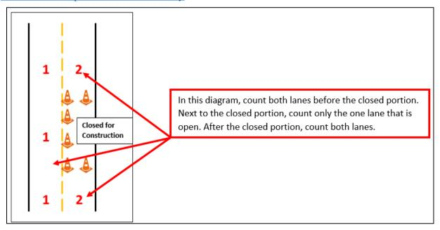
Figure 25. Example of counting lanes around a closed portion of the trafficway
