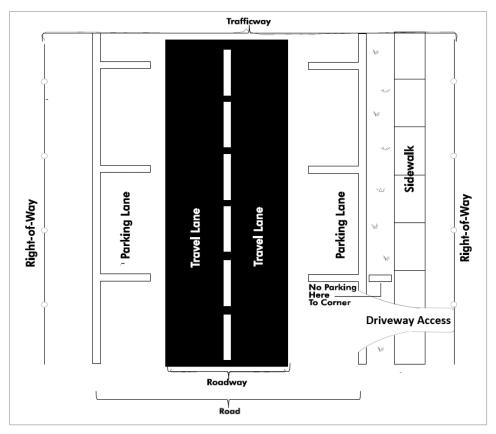
Figure 4. Diagram of a trafficway with parking lanes
