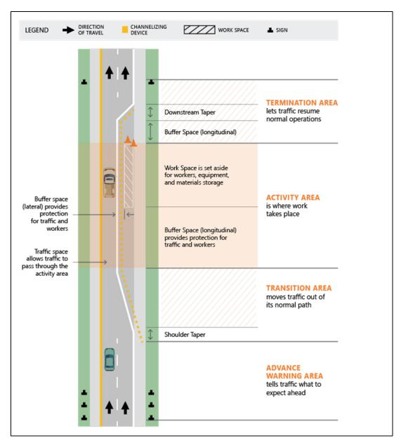
Figure 11. Diagram of a work zone area
