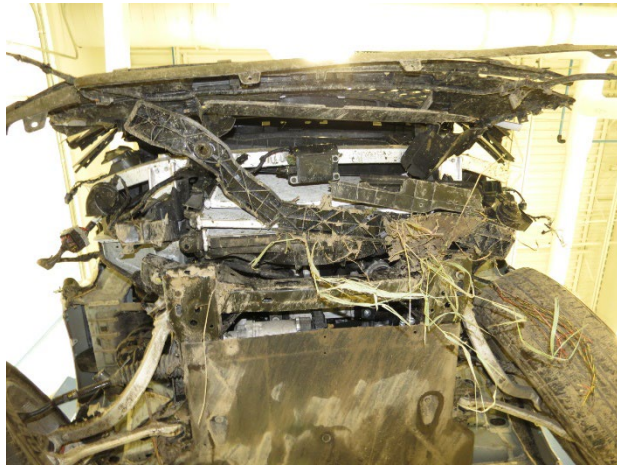
Figure 8. Undercarriage damage across the front of the Genesis
