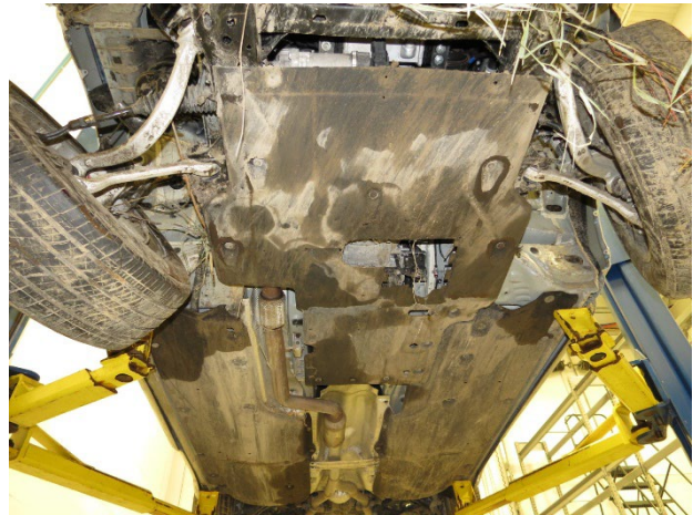
Figure 9. Undercarriage damage to the center and rear of the Genesis
