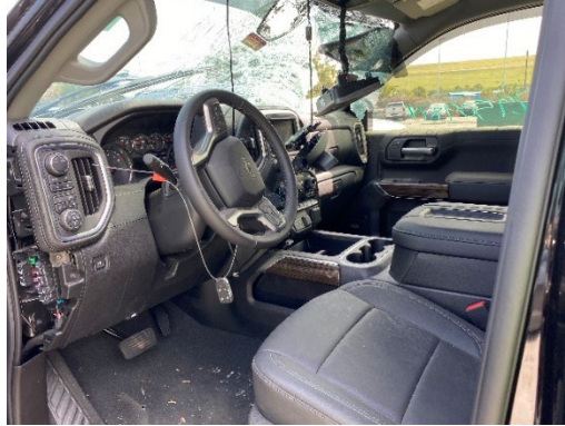
Figure 12. Oblique view of the driver's side showing the non-deployment of the driver's frontal air bags
