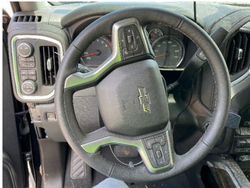
Figure 13. View of the steering wheel showing the non-deployment of the driver's frontal air bag
