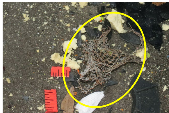
Figure 14. Closeup of mesh filter embedded into floor mat
