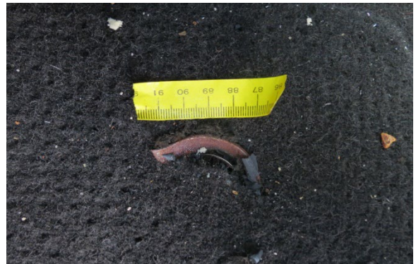
Figure 16. Inflator's horizontal divider embedded in floor carpeting
