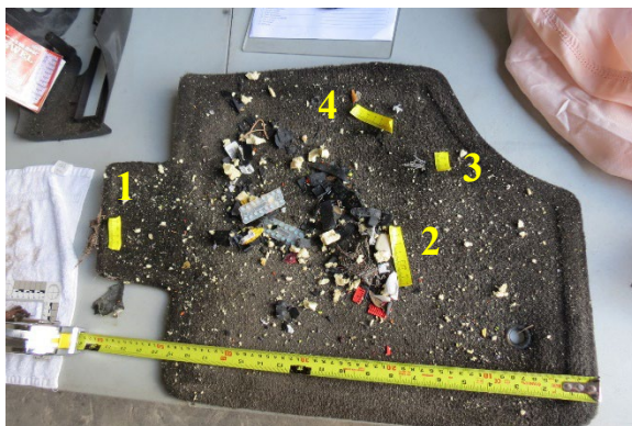
Figure 13. Inflator mesh filter (1, 2 and 3) and horizontal divider (4) embedded in the floor mat
