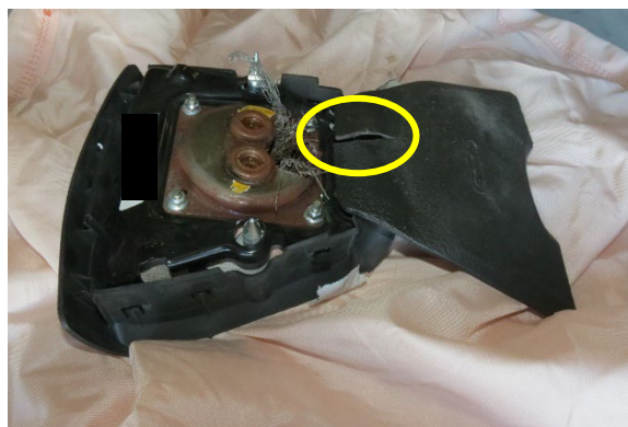
Figure 7. Cut on bottom flap of air bag module
