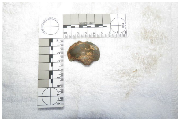
Figure 12. Ruptured fragment from stage 2 side of air bag inflator
