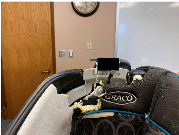
Figure 27. Front view of the damage to the CRS by the fence post
