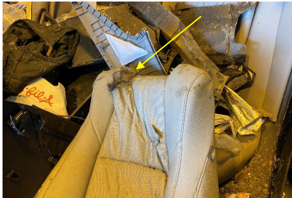
Figure 14. View of the driver's hair in the driver's seat back from intruding fence post
