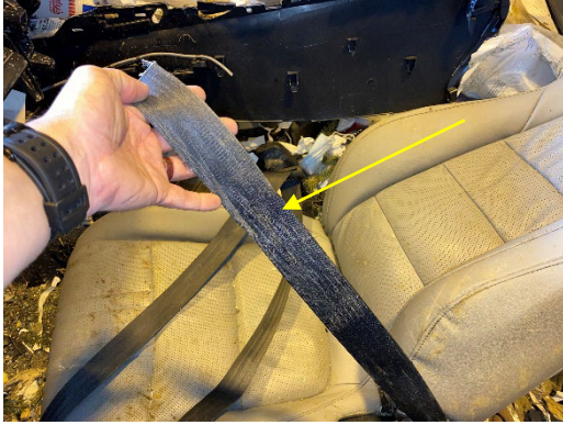
Figure 16. View of the driver's seat belt showing loading evidence from the B-pillar D-ring
