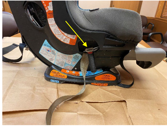
Figure 26. Right side view of the CRS showing the LATCH clip wedged under the metal routing bar
