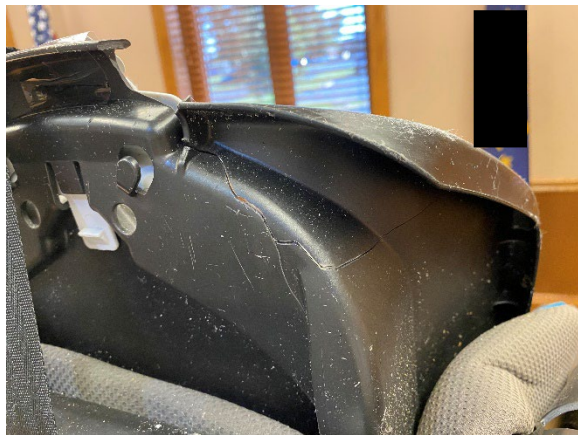
Figure 28. Rear view of the damage to the CRS by the fence post
