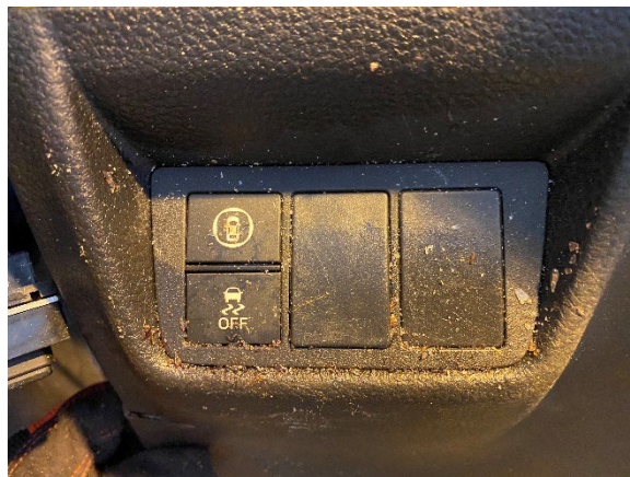
Figure 22. View of the crash avoidance system buttons located on the instrument panel left of the steering column
