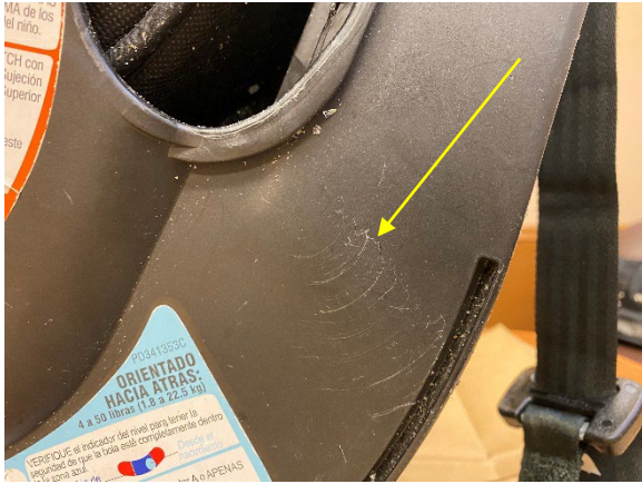
Figure 25. View of the left side of the CRS showing the front facing belt route stress damage
