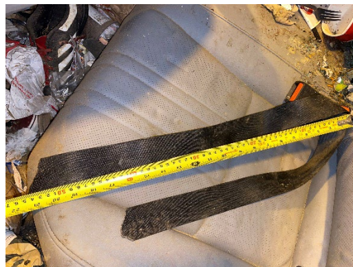
Figure 19. View of the second-row-left seat belt showing the extracting cuts
