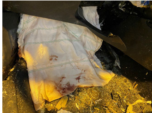
Figure 21. View of the deployed driver knee air bag in the Honda
