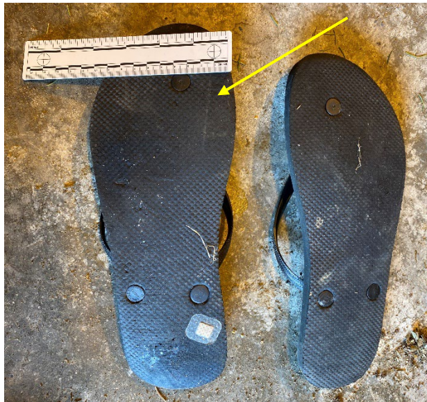
Figure 12. Driver’s sandals showing right sandal with an impression from the accelerator pedal
