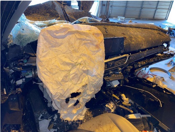
Figure 20. View of the driver's deployed frontal air bag in the Honda
