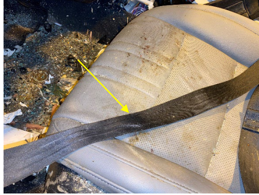
Figure 17. View of the driver's seat belt showing loading evidence
