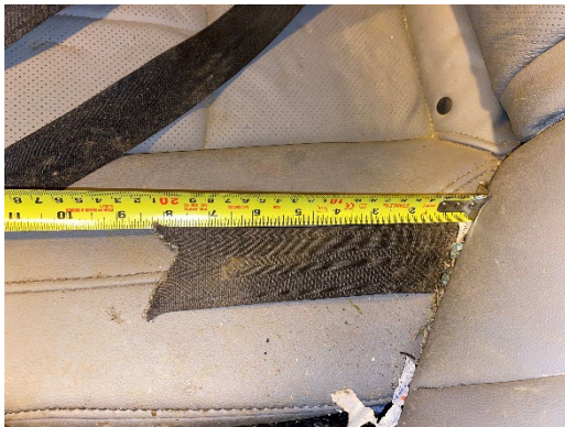
Figure 18. View of the second-row-left seat belt showing the extracting cuts
