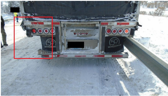
Figure 11. Back-plane damage, 2019 East trailer (police photo)
