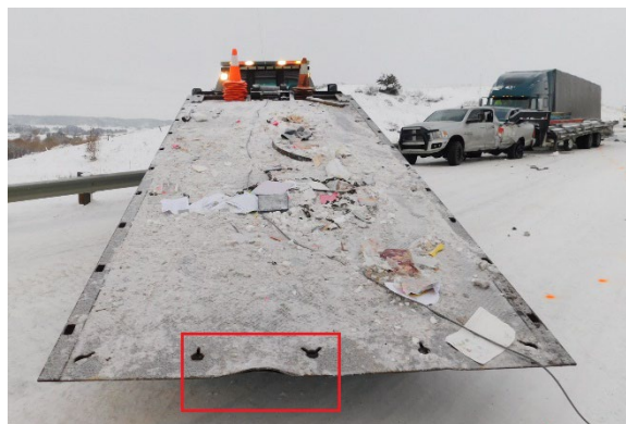
Figure 6. 2006 GMC TC6500, bed damage, looking southeast (police photo)
