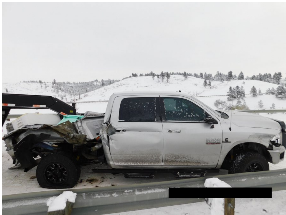
Figure 7. Right plane damage, 2016 Ram 3500 (police photo)
