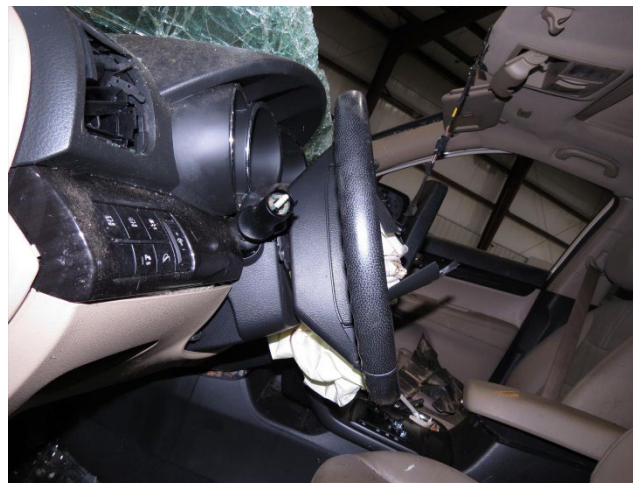
Figure 10. Compression of the steering column from driver loading
