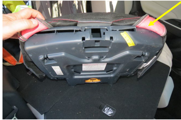
Figure 12. Separation of seating surface from the booster seat base
