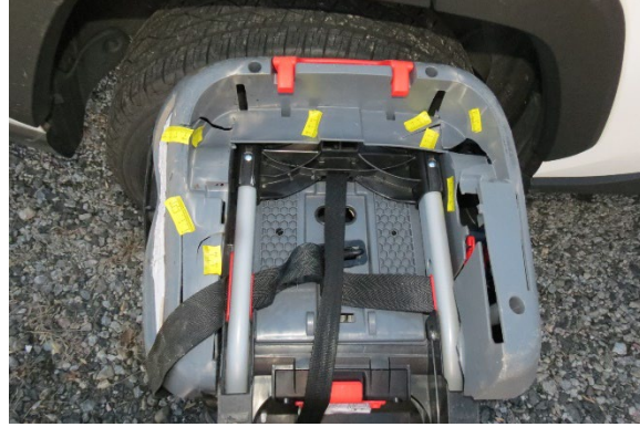
Figure 16. Broken and cracked plastic bottom of the second-row right CRS
