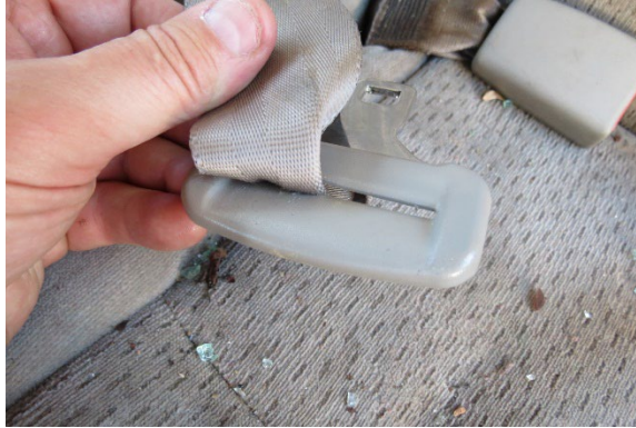
Figure 8. Second-row, middle seat pinched webbing and load mark on the latch plate belt guide
