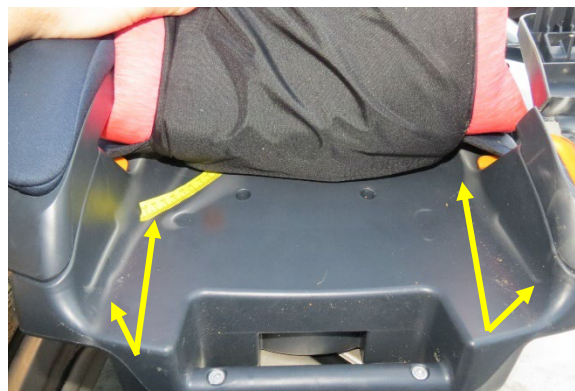
Figure 13. Stress marks on top of the booster seat
