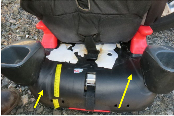
Figure 15. Front/top of CRS seat stress marks on the right and left sides
