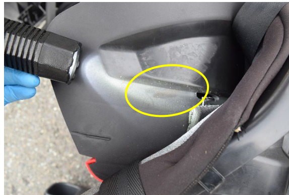
Figure 17. Scuff on the left exterior of the headrest
