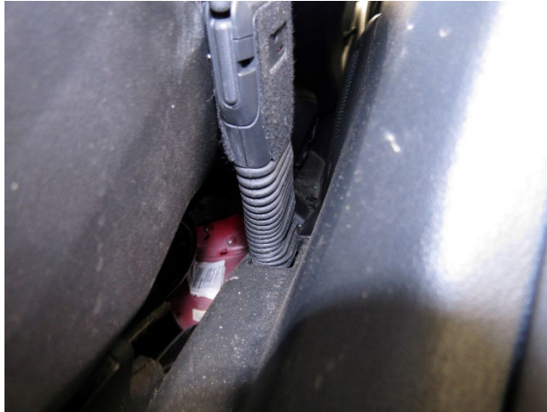
Figure 11. Driver's seat belt anchor showing signs of actuation
