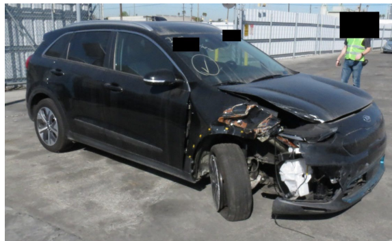
Figure 1. 2020 Kia Niro, front-plane damage
