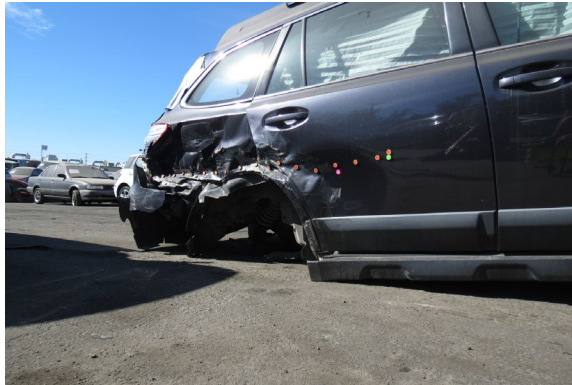
Figure 3. 2012 Subaru Outback, right-plane damage
