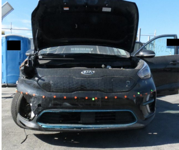
Figure 2. 2020 Kia Niro, front-plane damage
