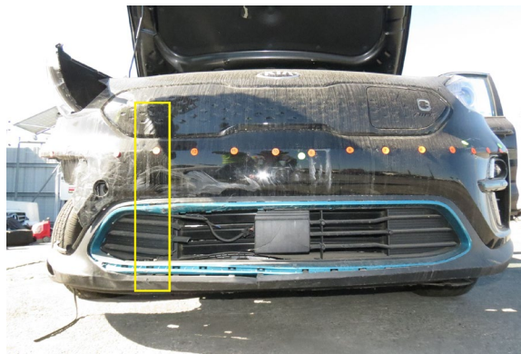
Figure 10. 2020 Kia Niro front-plane damage (pole impact highlighted)
