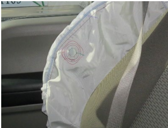
Figure 10. View of the front right occupant side seat-mounted air bag exhaust port
