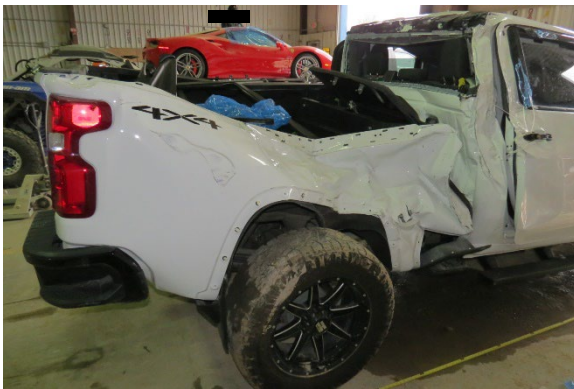
Figure 9. Right side damage from dead tree contact
