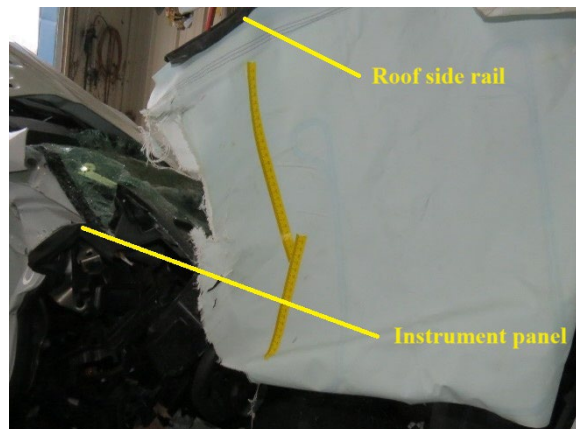
Figure 14. Damage to driver's IC air bag from tree contact (outboard side)
