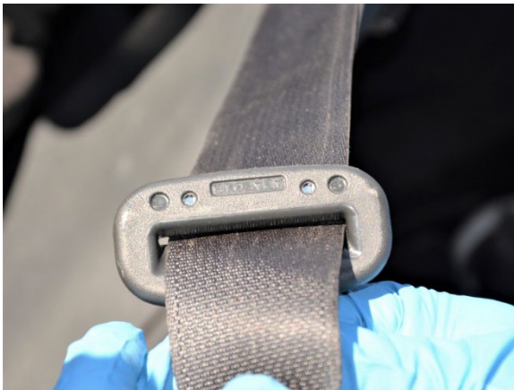
Figure 12. Second-row left latch plate and webbing
