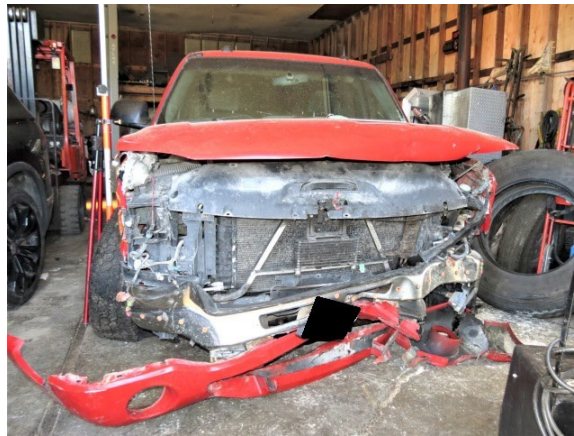
Figure 15. Front plane damage 2004 GMC Sierra
