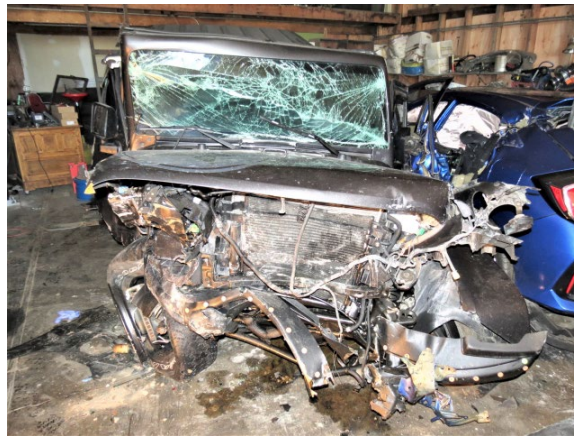
Figure 14. Front plane damage, 2018 Jeep Wrangler
