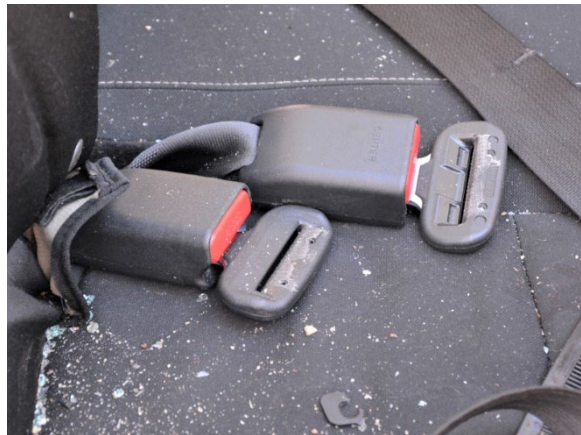
Figure 13. Second-row center and right latch plates and buckles
