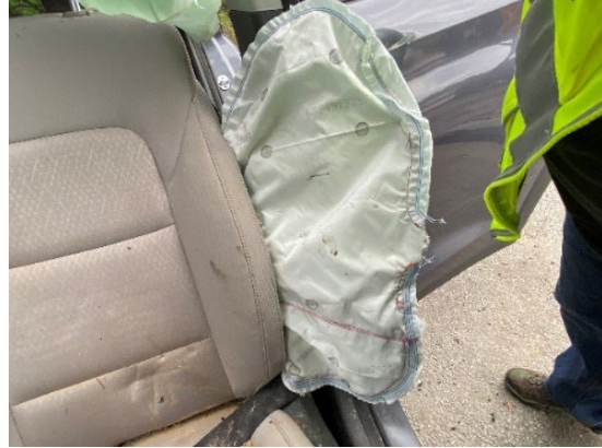
Figure 7. View of the driver's seat-mounted side impact air bag in the Hyundai
