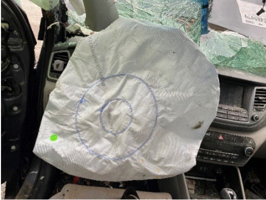
Figure 6. View of the driver's frontal air bag in the Hyundai
