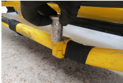
Figure 19. Fractured locking pin from the cot frame (placed back on frame for reference)
