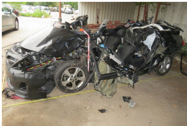
Figure 21. Event 1 involving the Toyota's left plane damage
