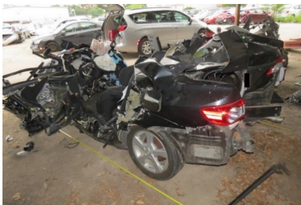
Figure 22. Events 4 and 5 involving the Toyota's left and rear plane damage
