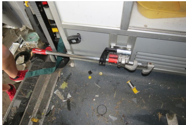
Figure 13. Rail clamp cot fastener system with fractured pin
