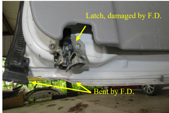
Figure 12. Left rear door latch (note bottom of door bent upward by rescue personnel to access latch)
