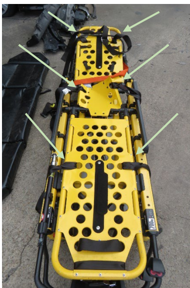
Figure 16. Cot mattress platform (note restraints anchored to the mattress platform)
