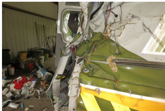
Figure 11. Right rear door hinge separation
