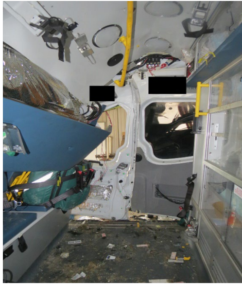
Figure 9. Intrusion damage to the right rear of the patient compartment
