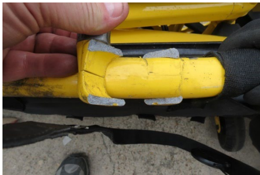
Figure 20. Fractured locking pin bracket
