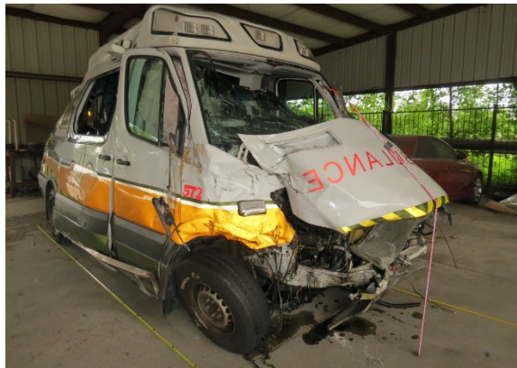
Figure 6. Front end and right-side damage
