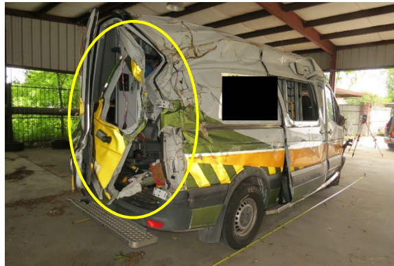
Figure 10. Right rear door separation
