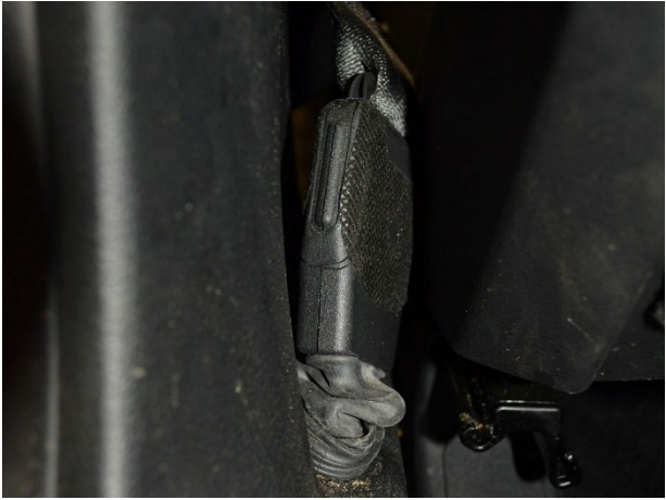
Figure 19. Driver's actuated anchor pretensioner
