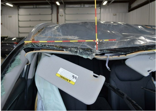
Figure 11. Crush damage to the windshield header
