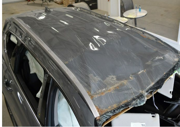
Figure 12. Surface abrasions to the roof
