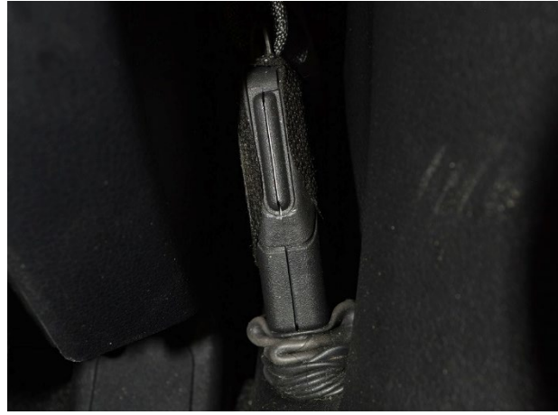
Figure 20. Front passenger's actuated anchor pretensioner
