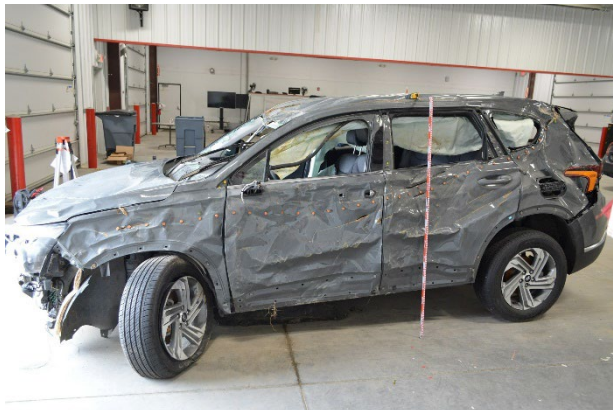
Figure 10. Left side of the Hyundai and the damage associated to Event 3
