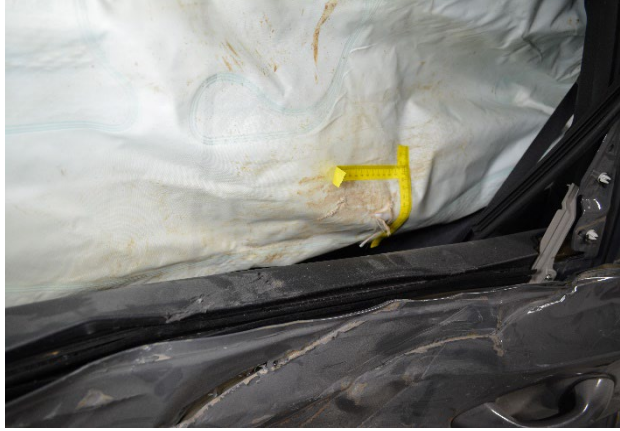
Figure 21. Exterior view of the left rear passenger's IC
