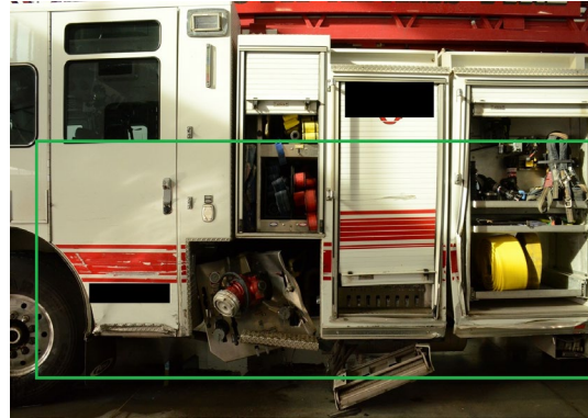
Figure 6. 2018 Pierce fire truck left-plane damage (fire department photo)
