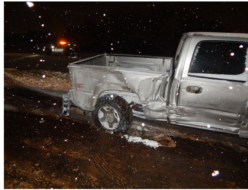
Figure 8. 2005 Chevrolet Silverado right-plane damage (fire department photo)
