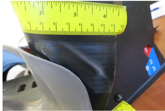
Figure 11. Left belt guide abrasions from webbing
