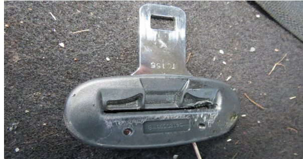
Figure 8. Load marks on latch plate belt guide, second-row-right seat
