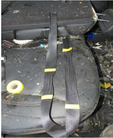
Figure 7. Second-row-right seat stretched and abraded- seat-belt-webbing
