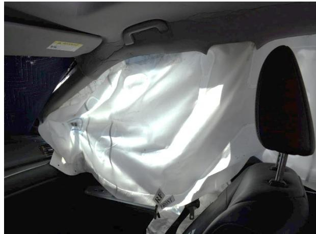
*Figure 19. Front passenger's IC air bag*
