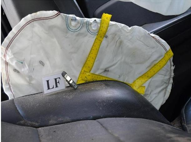
*Figure 16. Driver's outboard seat-mounted air bag*
