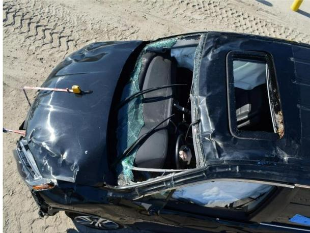
*Figure 7. Rollover damage to the left side*
