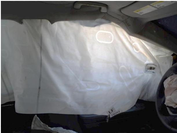
*Figure 18. Driver's IC air bag*
