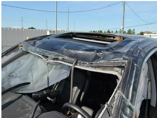
*Figure 8. Vertical intrusion to the windshield header during the rollover event*
