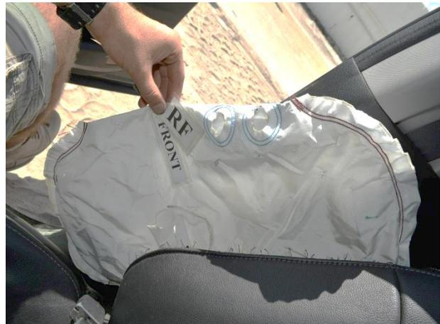
*Figure 17. Front passenger's outboard seat-mounted air bag*
