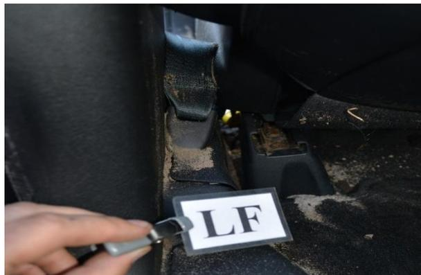
*Figure 13. Viewing the driver's actuated lower anchor pretensioner*
