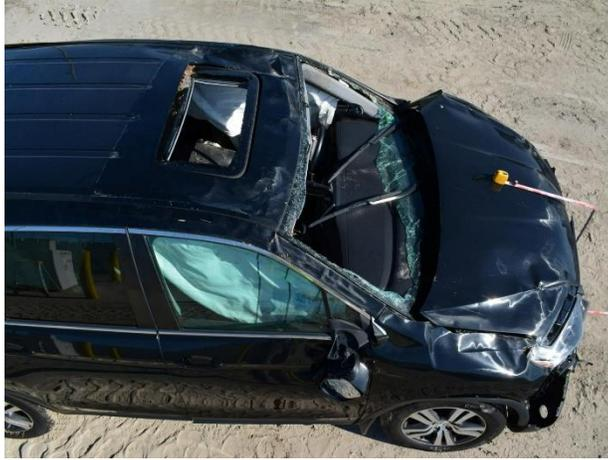
*Figure 9. Rollover damage to the right side*
