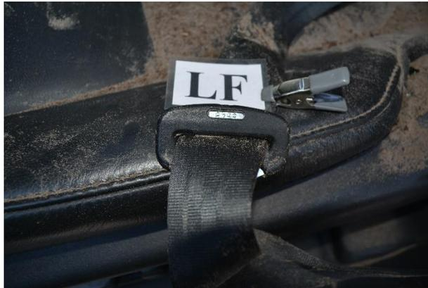
*Figure 15. Driver's latch plate with friction burns*
