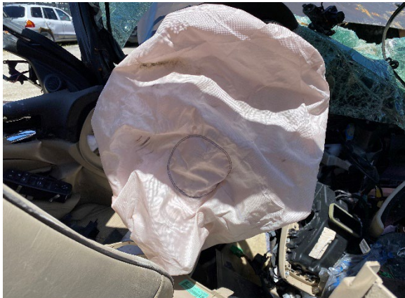
Figure 14. View of the driver's frontal steering wheel hub-mounted air bag
