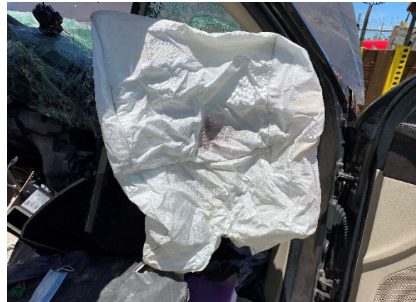
Figure 15. View of the deployed passenger's frontal air bag
