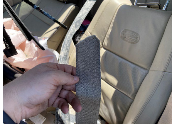
Figure 13. Close-up view of the extrication cuts of the driver's seat belt in the Jeep
