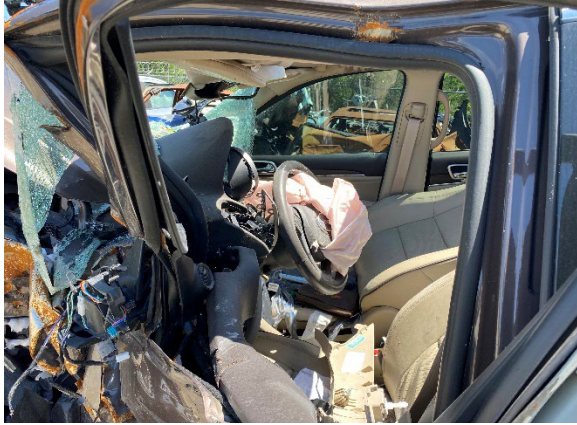
Figure 8. Lateral view of the Jeep's left A-pillar deformation
