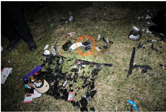
Figure 10. Image of the fractured sunroof glass at the Jeep's final rest location. Image provided by local law enforcement.
