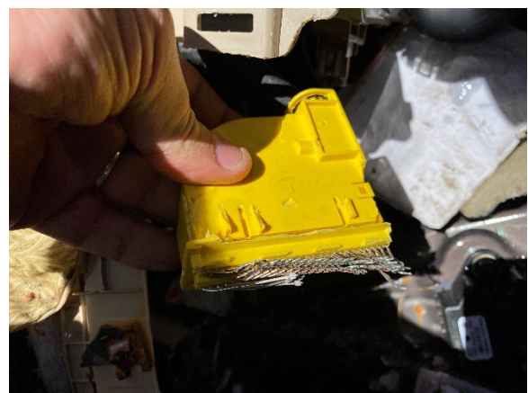
Figure 7. View of damage to the Jeep's EDR connector cable
