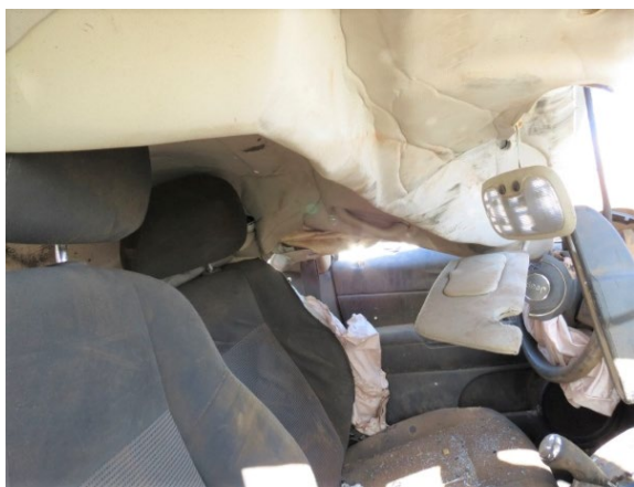
Figure 7. Interior damage, 2016 Jeep Compass
