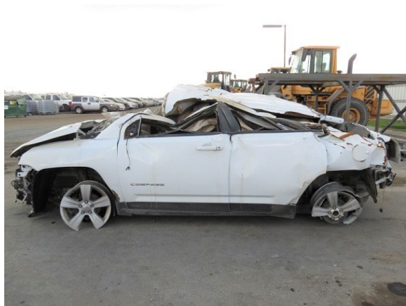
Figure 5. Rollover damage, 2016 Jeep Compass
