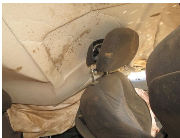
Figure 8. Interior damage, 2016 Jeep Compass
