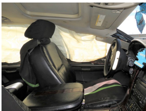
Figure 8. Deployed left IC air bag, the 2008 Cadillac Escalade
