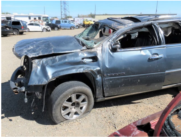
Figure 5. Rollover damage, left and top planes, the 2008 Cadillac Escalade
