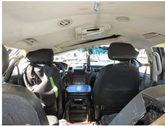
Figure 7. Vertical intrusion, the 2008 Cadillac Escalade
