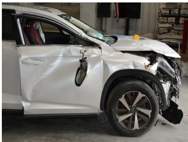
Figure 9. Damage to the right A-pillar and right front door from Event 4
