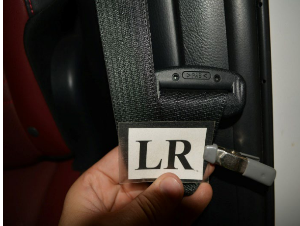
Figure 15. Left rear passenger's latch plate void of friction evidence
