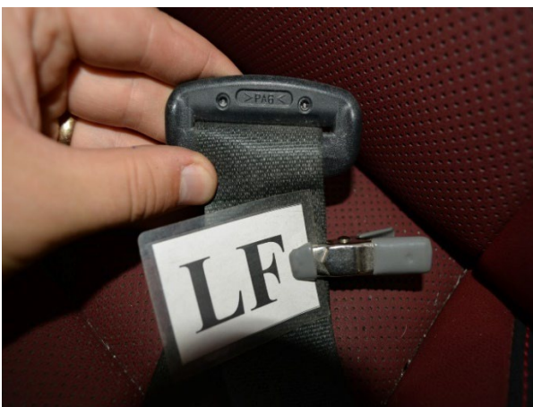
Figure 13. Driver's latch plate with friction burns evidence
