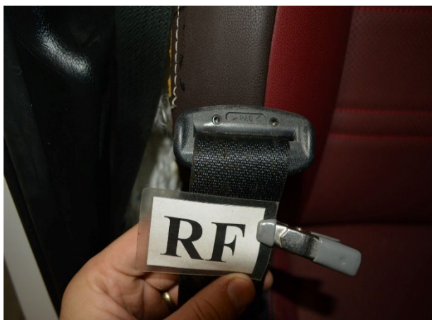
Figure 14. Front passenger's latch plate with friction burn evidence
