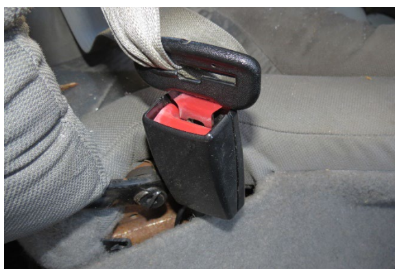
Figure 11. Jammed seat belt webbing in driver's latch plate (found buckled at time of the SCI inspection)
