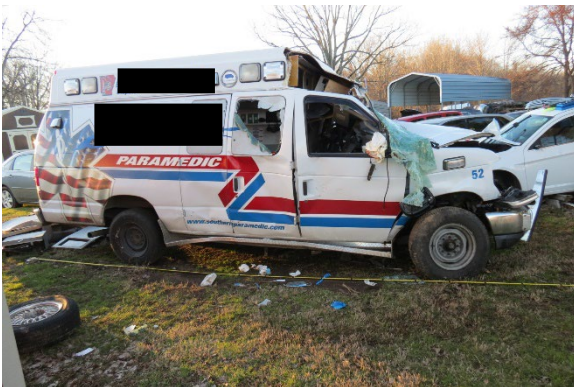
Figure 7. Minimal rollover damage on the ambulance's right side
