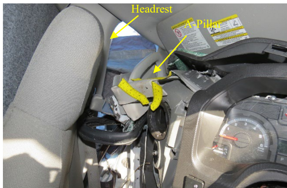
Figure 10. Longitudinal intrusion and contacted left A-pillar
