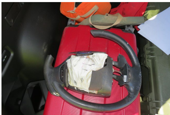
Figure 13. Cut steering wheel rim and air bag module, found at crash scene
