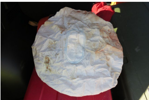
Figure 12. Deployed driver's frontal air bag
