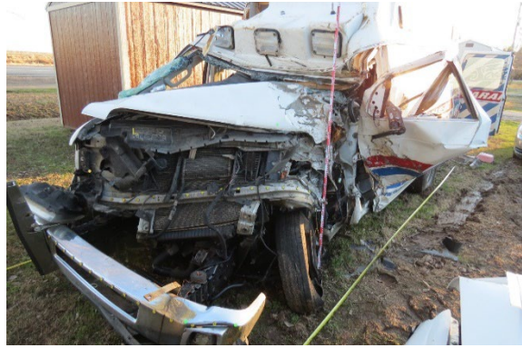
Figure 6. Front plane damage on ambulance
